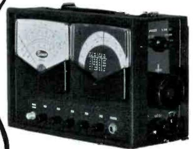
Dimensions: 5 1/4" x 11 1/4" x 7 3/4" □ Weight: only 10 lbs. including batteries □ Sensitivity: 5 microvolts minimum readable signal or 60 m/v full scale with sensitivity control at maximum □ Selectivity: all spurious responses including image more than 80 db down, 4.5 Mc/s or more away from selected frequency □ Battery Life: 180 hours continuous or better than 3 hours per week for one year.
