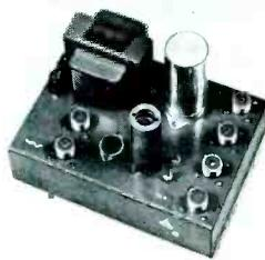
**Low band bridging amplifier, Model BA-1-4.** Low output loss, transformer coupling on output, variable tilt. Gain: 3 db at Channel 6. Self-contained power supply. Output: 45 db, Channel 6. Designed to drive 4 sub-trunk lines. Net: \$80.00.
