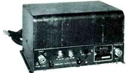
**Automatic gain control** for use with CATV broadband amplifiers, Model MAC. For use with any broadband VHF amplifier having more than 16 db gain and producing an output between 0.6 volts and 2.5 volts per band. It will maintain the output at a constant level (less than 1 db change in output level for a 10 db change in input). In addition to providing AGC the MAC can deliver up to 10 db additional gain. Net: \$121.50.
