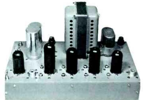
**Low band trunkline amplifier, Model LRA-40C.** Operates as low band VHF repeater. Incorporates ALC circuit. Gain at Channel 6: 40 db. Tilt: 7 db (Channel 6 over Channel 2). Noise figure: 7.5 db. Maximum output level: +50 dbmv (single amplifier—Channel 6). Uses 10,000 hour tubes and regulating transformer. "Sister" amplifier to Entron's HRA-400 for expansion to all-band operation. Net: \$299.25.
