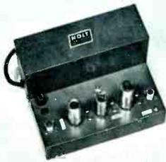
**Low band line amplifier, Model LBB-MAN-50.** 4 to 9 db variable tilt. Manual gain. Output: 45 db. Gain: 50 db at Channel 6. Utilizes electronic regulation. 75 ohm input and output. Self-contained power supply. Net: \$150.00
