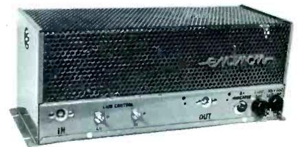
**Broadband amplifier, Model FA-283.** Covers Channels 2 thru 13 plus FM. Noise figure 8 db. Separate high and low band gain controls. Gain: 38 db high band and low band, 32 db FM. 75 ohm input and output impedance. Net: \$149.25.
