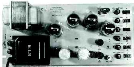
**Regulated power supply, Model PSR-3.** Output 160 vdc at 800 ma. maximum regulated. 6.3 vac at 20 A. maximum unregulated. Minimum load 0 ma., regulation  $\pm 0.3\%$ . Takes 8 3/4" of rack space in 19" standard rack. Tubes: (1) 5651, (4) 6080, (1) 5654. Net: \$300.00.
