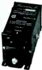
**Pacemaker 35 db TV/FM amplifier, Model PM-2.** Broadband amplifier with low band gain of 35 db and high band gain of 30 db. Noise figure 6 db average; maximum output 2 volts per band. Separate gain controls for each band allowing up to 10 db change. PNS.
