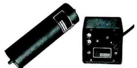
**Single-channel preamplifier, Model AP-3.** Designed for cable powering or can be battery powered. Power supply can be located up to 600 feet from pre-amp. Low noise figure on both high and low band. Gain: 40 db (low band) and 35 db (high band). 75 ohm input and output impedance. For storage battery operation, unit requires 9 vdc at 18 ma. Net: \$70.00.
