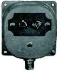
**MTU-372**—Matching transformer for indoor service. Surface mounting. Flat response over the entire UHF band. Insertion loss: .6 db at 470 Mc and 1.2 db or less at 890 Mc. F-61 connectors. PNS.
