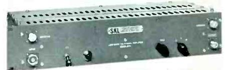
**Low band amplifier, Model 211C.** Covers 10-100 Mc. Gain: 33 db at 88 Mc. Choice of gain control, either manual or automatic using external 830 ALC or thermatic using external 832A Thematic Gain control. Regulated, self-contained power supply. Cup core type transformers at the input and output provide excellent impedance match to the line. Rack or cabinet mounting. Net: \$328.00
