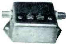
**FM TAP** Model IWD-1 TV-FM is a non-resistive attenuator network for use in tapping off from the feeder thurline to individual FM subscribers. Complete AC isolation, only 0.5 db thurline attenuation, FM tap off band 88 to 108 mcs.
