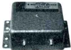
**FOUR-WAY LINE DIVIDER** 20 db isolation between outlets. Completely shielded eliminating pick up. Matched 75 ohm input, four 75 ohm outputs. 6 db loss per output, 7 db thurline loss. MF-61 connectors, with five MF-59 male connectors supplied.
