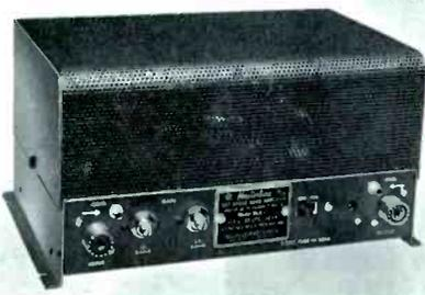
The high gain, high output VHF amplifier is especially designed to overcome coaxial cable and distribution system losses in television and FM master antenna systems without signal degradation. Net price on the MLA-FM is \$101.00 and is available with ruggedized tubes at slightly higher cost.
