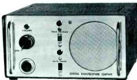
radio, known as the FM-120. The FM-120 is a compact 60 watt input FM transceiver designed to operate in the 150-174 Mc band. It includes such features as a dual power supply, 115 VAC or 12 VDC, a size of 4 1/2" x 8" x 10 1/2" that permits installation in the smallest of places and the exclusive "Snap-Rak" mounting which allows replacement and interchange of units in 30 seconds without the need of any tools. The FM-120 is designed as a quality unit to provide reliable communication at low cost.
