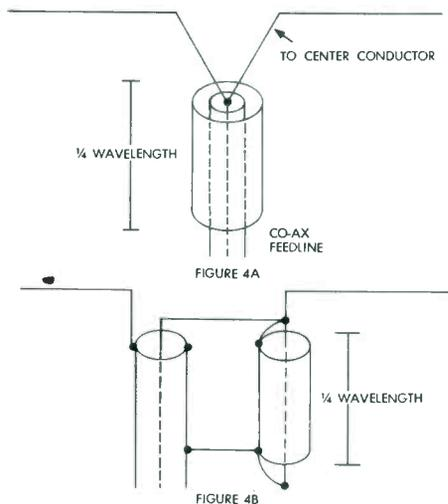
Note that in Figure 4 A the bottom of the cylinder is connected to the coax braid. It is a quarter-wave in length so that at the open end, it is a high impedance. The center conductor of the coaxial line is already at a high impedance with respect to ground and the same is true of Point X. We connect the balanced antenna to the center conductor and to Point X and our problem is solved.
