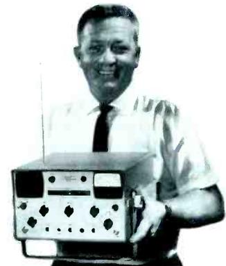
The unit operates from 117 vac, 230 vac or 12 vdc, or an optional rechargeable battery pack.
