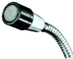
The unit is compact (2-41/64 inches long, 1-23/64 inches diameter), and its voice-response peaked for base station installations. The unit has a low impedance permitting unusually long cable runs without adverse effects on response characteristics or levels. Frequency response is 40 to 10,000 cycles with a rising characteristic to 4,500 c.p.s. Price on the new microphone is \$32.50.
