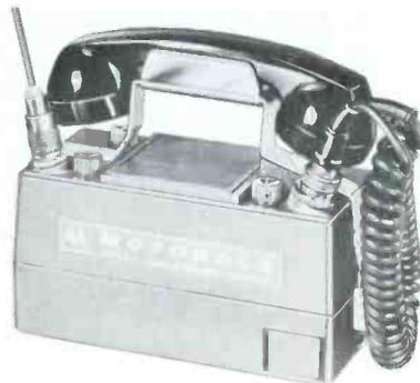
The new compact hand-carried sets are ready to operate at only 6 pounds carry-away weight. The sets are available in the 5 and 1.4 watt versions for 25 to 54 megacycles and 3 and 1.4 watt versions for 144 to 174 megacycles. Receiver sensitivity is 0.5 microvolts in the low band versions, 0.3 microvolts in the high band version. The radios can be powered from a single rechargeable nickel cadmium battery, and can be equipped with Motorola's Private-Line selective calling system.
