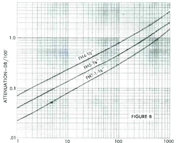
Fig. 8 Attenuation curves, 1/2", 7/8" and 1 5/8" foam Heliac.
