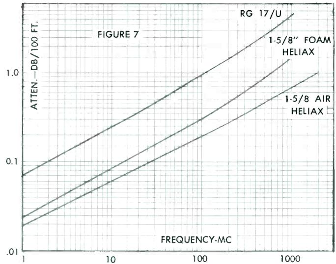
Fig. 7 Attenuation curves, 1 5/8" foam and air dielectric Heliac.
