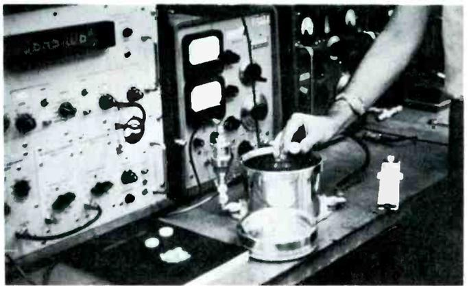
Fig. 2 Laboratory setup for measuring loss in dielectric.
