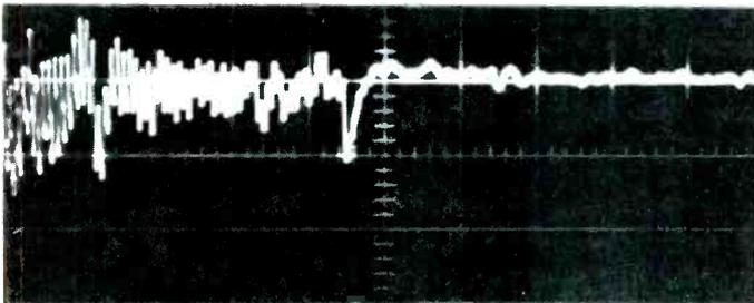
Fig. 5 Pulse measurement, RG8 on left, 1/2" foam Heliac on right.
