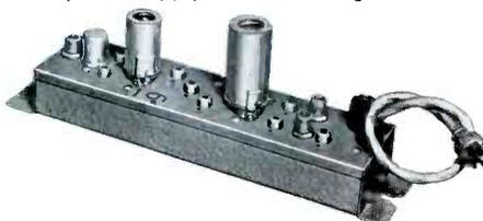
**Single-channel amplifier, PMA series.** Consists of single-channel strips, Models PMA-2 through
