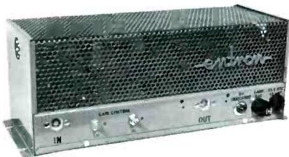
**Broadband amplifier, Model FA-283B.** Covers channels 2 thru 13 plus FM. Noise figure 8 db. Separate high and low band gain controls. Gain: 38 db high band and low band, 32 db FM. 75 ohm input and output impedance. Built-in power supply. Input and output impedance, 75 ohms. Price: \$99.50.
