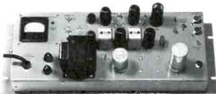
**FM transmitter, Model FMT-1100.** Accommodates multiplex or monaural audio input. FM RF output. Standard 75 usec. pre-emphasis. Factory aligned to any one of the 26 FM channels. Maximum output level: 0.2 volts. Level control range: 25 db. Stereo channel separation: 35 db. Hum and noise: down 55 db at 75 kc deviation. 10,000 hour tubes.
