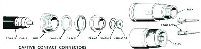
Superior's Captive Contact Connectors eliminate the "pullouts" that cause blank screens by making positive never-fail contact between lengths of coaxial cable to maintain service. Designed to mate electrically and mechanically with #4920 and #4930 "Cell-O-Air" coaxial cable with "Coppergard" shield, Superior's captive contact connectors assure full-system compatibility.
