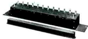
**Tunable filter, Model DBR-26.** Provides two 40 db reject bands, 3.5 Mc wide on each side of a channel. Each notch is tuneable over the complete range. As a single notch filter, typical adjustment provides a 25 db, 6 Mc notch; a 75 db, 1 Mc notch; or a 600 kc notch width having 90 db minimum attenuation. Net: \$277.50.
