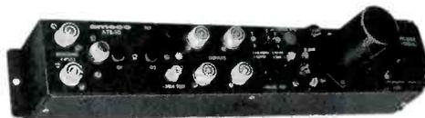
**Transistorized all-band bridger amplifier, Model ATB-11.** Two 40-220 mc inputs; four 40-220 mc outputs. 15 db average gain with maximum output of 45 db. Noise figure 10 db measured at 220 mc. Tilt control, 15 db. AC/DC cable powered, regulated power supply. 7 5ohms—input and output impedance. Cascadeable. Pole or strand mounting. PNS.
