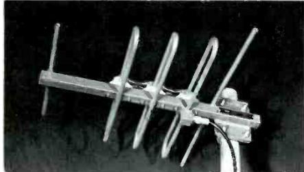
Multi-channel 5-element yagis, Y-53 series. 50 to 500 mc with models broad-banded to cover wide ranges within TV and communications spectrum. Especially applicable for multi-channel use for either high or low TV channels. Construction features include 1 1/2" square heliarc welded crossarm with 1/2" diameter elements reinforced with 5/8" sleeves. Gain at channel 2 is 7 db; at channel 6, 7 db and 7.5 db at channel 13. Three driven elements. Hermetically sealed terminal boxes. 50 ohm impedance.
