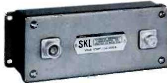
**Crystal-controlled VHF to VHF converter, Model 276.** Operates from 28 vdc. Matched input and output. Converts any VHF channel to any other VHF channel with single or double conversion. Gain: unity to + or -3 db. Rack or wall mounting. Completely transistorized unit. Net: \$280.00
