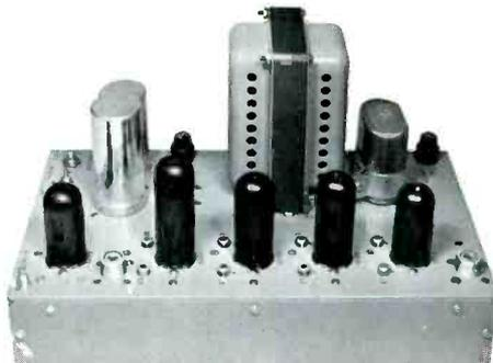
**Low band trunkline amplifier, Model LRA-40D.** Utilizes 10,000 hour input tube and 10,000 hour DC amplifier tube. Gain control range, continuously variable 0 db to full gain of amplifier. Average gain, 35 db. Output, plus 52 dbmv. Mounts any position on pole crossarm. Price: \$170.00.
