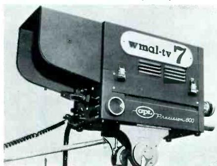
**Precision 800 series.** Studio type camera chain for open or closed circuit use. System includes viewfinder and portable or rack-mounted camera control unit (CCU). Designed to accept external EIA pulses or operate independently from its internal sync generator. 525 line system interlaced 2:1.
