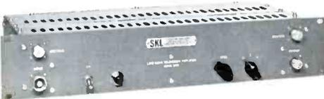
**Low band amplifier, Model 211C.** Covers 10-100 Mc. Gain: 33 db at 88 Mc. Choice of gain control, either manual or automatic using external 830 ALC or thermatic using external 832A Thematic Gain control. Regulated, self-contained power supply. Cup core type transformers at the input and output provide excellent impedance match to the line. Rack or cabinet mounting.
