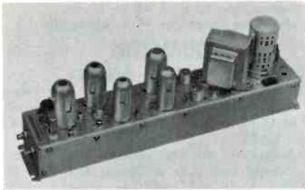
plus sound carrier which may be modulated by any audio source. Audio carrier is 4.5 mc above video frequency (TV Standards) Output impedance is 75 ohms. Net: \$174.25.
