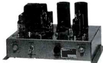
**Low band AOC line amplifier, Model ABB-14.** Covers low band and FM. Gain of 35 db; maximum output of 48 dbmv. Tilt control, 2-5 db. Gain control. Line powered. Ruggedized tubes. Cascadeable with 14 units at plus 48 dbmv. 75 ohm. Price: \$135.00.
