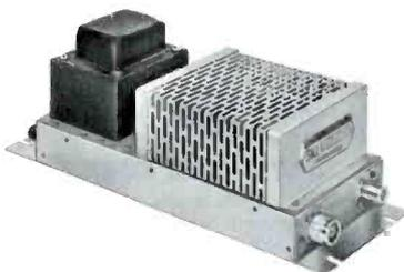
**All-band line extension amplifier, Model 209B.** Frequency range: 20 to 216 Mc. Gain: 27 db at 216 Mc. Cabinet mounting. Noise figure under 14 db over entire band. 10 db manual gain control. Low cost distribution amplifier with mainline dependability. 115 vac powered.
