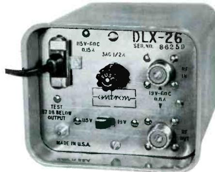
**Low band line extender amplifier, Model DLX-26.** Extends lines up to 2000 additional feet, using low-loss cable, or 1000 feet with standard cable. Average gain, 20 db. Maximum output, 41 dbmv. Noise figure, 8 db. Self-contained power supply; local or remote powered. 10,000 hour input tube. Mounts built-in or with mounting bracket Model QAB. Price: \$80.00.
