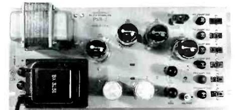
**Regulated power supply, Model PSR-3.** Output 160 vdc at 800 ma. maximum regulated. 6.3 vac at 20 A. maximum unregulated. Minimum load 0 ma., regulation  $\pm 0.3\%$ . Takes 8 3/4" of rack space in 19" standard rack. Tubes: (1) 5651, (4) 6080, (1) 5654.
