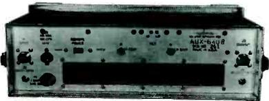
**Distribution line amplifier, Model ABX-640B.** 32 db gain. Maximum output 46 dbmv. Tilt control: low band plus 1 to minus 2 db; high band plus or minus 1 db. Gain control range, 32 db for low band, 20 db for high band. Self-contained power supply remote powered. 75 ohm. 10,000 hour input tubes. Mounting clamp for strand suspension. Price: \$170.00.
