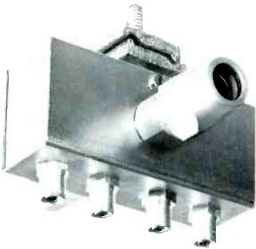
**Directional coupler, Model DT-4.** Four taps. For providing matched, isolated taps with directivity in distribution lines. 50 - 220 mc. 75 ohm. More than 30 db isolation. 0.7 db insertion loss. Loss per output 17 plus or minus 1 db. VSWR less than 1.1. Available with most connectors used in CATV. PNS.
