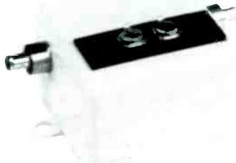
**OF-320—FM subscriber connection device.** Surface mounting. Ivory finish. FM tapoff attenuated 20 db. Push-on thru line fittings. 75 ohm input (thru line) and 300 ohm output (FM).
