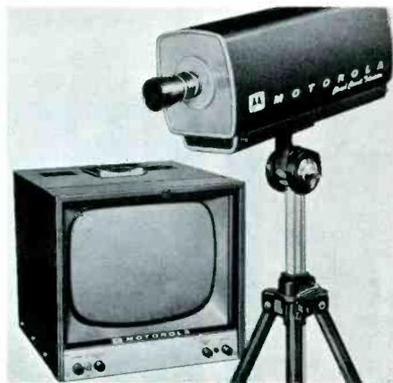
Complete line of closed circuit television cameras including transistorized indoor camera in aluminum case with 650 lines horizontal resolution. Motorola also has all-weather cameras with low height and sloping sides to minimize wind vibration.
