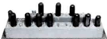
**High VHF to low VHF converter, Model CHL-D.** Converts any high band channel to any low band channel. Utilizes ALC system referenced to video carrier and a sound carrier level control. ALC will maintain output within plus 0.5 db for input variations of 10 db. Crystal controlled oscillator. 10,000 hour tubes. Gain: 60 db. Stability: plus or
