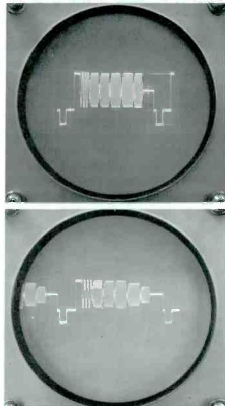
Figure 4. Multiburst signal consists of consecutive "bursts" of ascending frequencies, all transmitted at reference white level (A). Changes in frequency response show up as variations in relative amplitude of different frequencies (B). Note frequency roll-off at upper frequencies.
