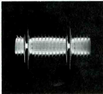
Figure 7. By passing staircase with subcarrier through a high-pass filter, low-frequency steps are removed, leaving only subcarrier. Variations in amplitude reveal differential gain more clearly than in original unfiltered form (Figure 6).
