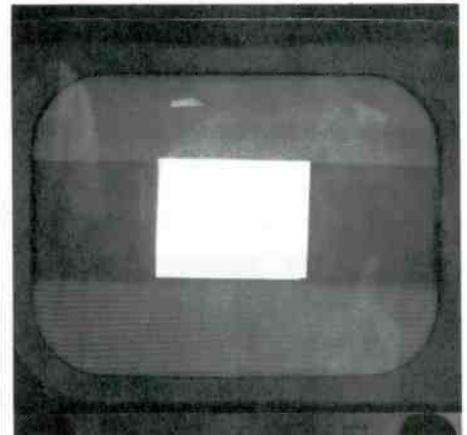
Figure 8. Streaking of picture is caused by poor low-frequency response. Note that relative duration of brightness values determines the amount of visible error in picture at left. At right is a typical window signal as it appears on the picture tube when the same amount of low frequency error is present.
