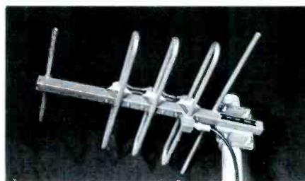
**Multi-channel 5-element yagis, Y-53 series.** 50 to 500 mc with models broad-banded to cover wide ranges within TV and communications spectrum. Especially applicable for multi-channel use for either high or low TV channels. Construction features include 1 1/2" square heliac welded crossarm with 1/2" diameter elements reinforced with 5/8" sleeves. Gain at channel 2 is 7 db; at channel 6, 7 db and 7.5 db at channel 13. Three driven elements. Hermetically sealed terminal boxes. 50 ohm impedance.
