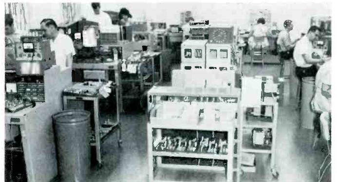
All Ameco products are subjected to close scrutiny in the Test and Alignment section before leaving the production plant.
