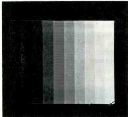
Figure 5. Typical staircase test signal as shown on the "A-Scope," and how it appears on picture monitor. Note that each step represents a shade of light. When applied to system, each step is equal in amplitude. Non-linearities in system are revealed by compression or expansion of individual steps or parts of waveform.
