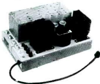
Its matched single input terminal allows the LHD-404R to be fed from a directional coupler or from the end of
