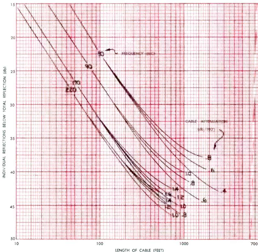
FIGURE 1. Relationships of total reflected signals to individual reflections at each discontinuity.
