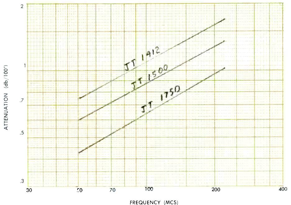
FIGURE D. Attenuation characteristics of aluminum sheath coaxial cables.
