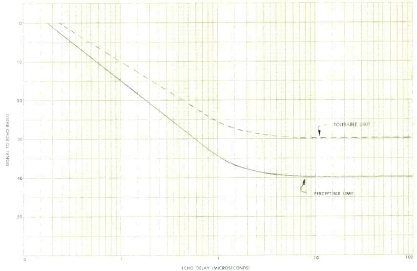
FIGURE A. Approximate tolerances of echo amplitude as a function of echo delay.
