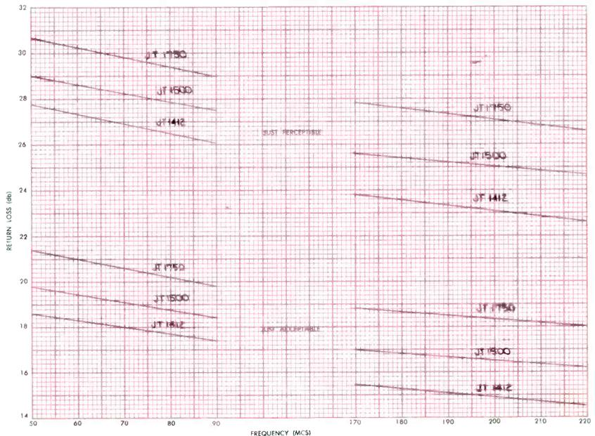
FIGURE 3. Return loss VS. Picture degradation
