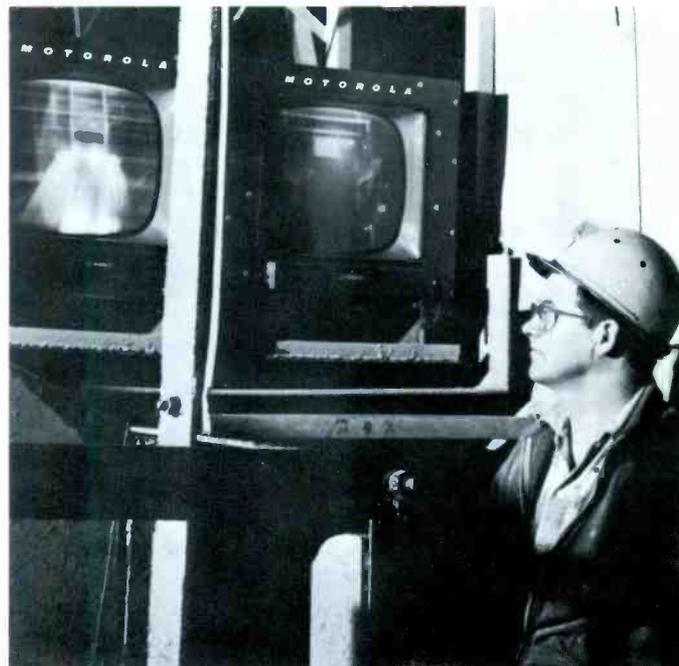
Hoist operator at the Southwest mine watches dumping of skips by means of closed-circuit television system.
