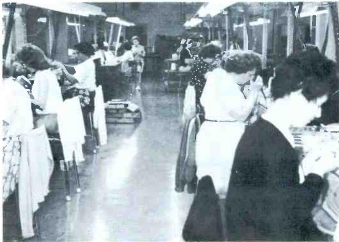
Entron's 250 feet of specially designed, well lighted assembly benches utilize air presses, riveting machines, air presses, miniature spot welders, induction beaters and drill presses. Special tooling is designed and fabricated in Entron's tool and die shop.
