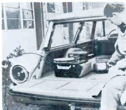
TV technician Dean Hilleman operates portable recorder on tailgate of station wagon used as mobile distribution center. Tape is used for playback into a Fontana school's antenna system through audio/video RF modulator.
