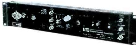
The Model TBA-1 is a bridging amplifier, designed to establish four feeder lines at main amplifier locations. It provides at least 14 db gain to each feeder line. Maximum output capability is 40 dbj for twelve channels. Response flatness is plus or minus 0.5db.
