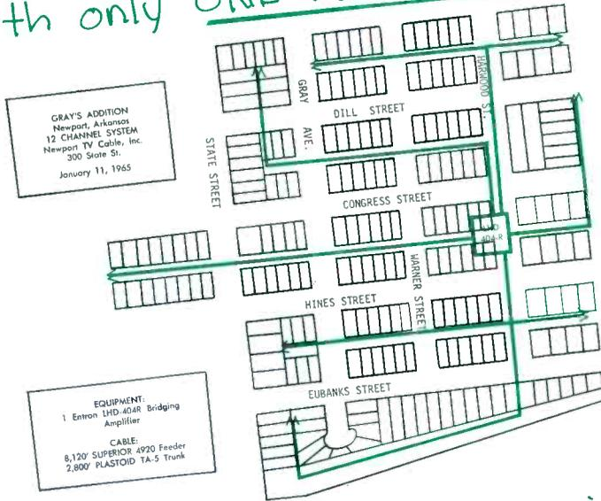
Please note that we have energized over 8,000' of FEEDER, and we are maintaining 20 db of signal at Channel 13 on each termination, delivering 9 TV Channels and 6 FM Channels.
