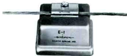
The new unit is designated as Model E-1. With its strand mounting feature and weatherproof design, it is installed at any point where TV and FM signals require amplification. The unit also employs silicon semiconductors and is powered by an Entron remote power transformer through the coaxial cable.
