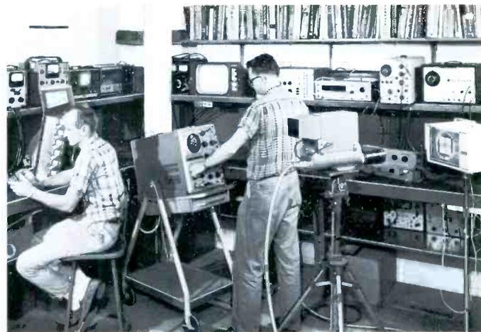
Engineer at left is setting Slave Reader for non-duplication switcher while engineer at right tests EIA camera chain.
