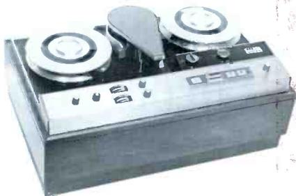
Ampex's home table-top model video tape recorder is approximately the size of a conventional audio recorder. It can be connected to any home television receiver with special connection components. The components will cost approximately \$25 installed.
