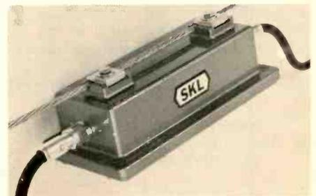
The nominal gain is 22 db at 216 mc, with a 7 db slope across the 54 to 216 mc band. Manual gain and tilt controls complete the compensation for the average cable losses encountered in feeder lines. Low noise and cross-modulation allow the Model 263 to be used even at the most remote ends of a distribution system.
