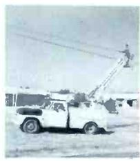
As cable television systems grow larger and enter larger urban markets, mechanized construction and maintenance equipment is of increasing importance to CATV'ers. Utility vehicles are the most significant tools used in construction and maintenance, from the standpoint of both function and cost. For this special staff report, see page 36.
