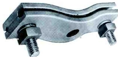
One groove accommodates insulated stranded support members of 1/4" and 5/16" diameters. Flip it over and the other groove accommodates insulated solid support members of .109", .134" and .148" diameters. Installed with 1/2" or 5/8" standard through-
