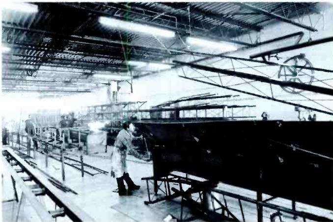
Tropo-scatter antennas are prefabricated in the Ajax, Ontario plant.
