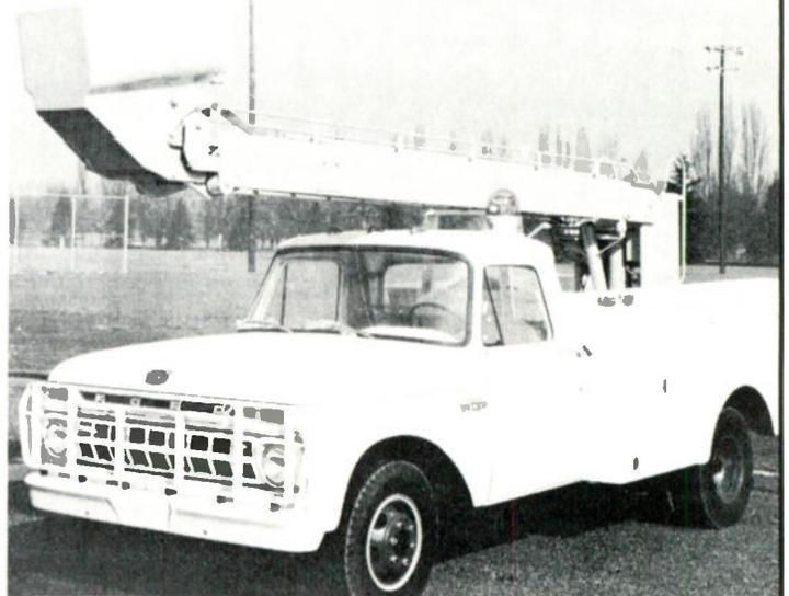
The EME is designed for any type of maintenance work. Choose from 4 models with extended platform heights of 26' to 35'. Four types of work platforms and baskets are available. Looking for a self-contained unit? The HALLINE EMH is your answer. Completely self-powered by a 9 h.p. gasoline engine housed in ladder base. Equipped with 110 A.C. outlet for use of electric power tools. 3 models available, 26'6" to 35'. CATV's best buy in self-contained ladders!
