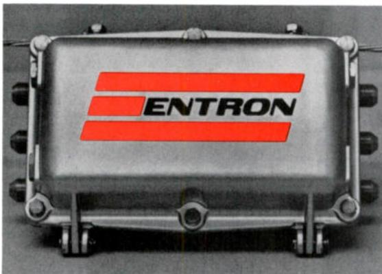
**1** Modular Trunkline Amplifier R-6T—Operational gain is 25 db. ALC, switching input pads, full-wave 30-v ac power supply. Remote-powered.
