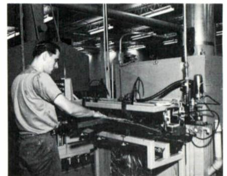
*Loosely assembled helical-wire subassembly pass under a cascade of liquid adhesive, then enter the drying oven where they are bonded into permanent assemblies.*
