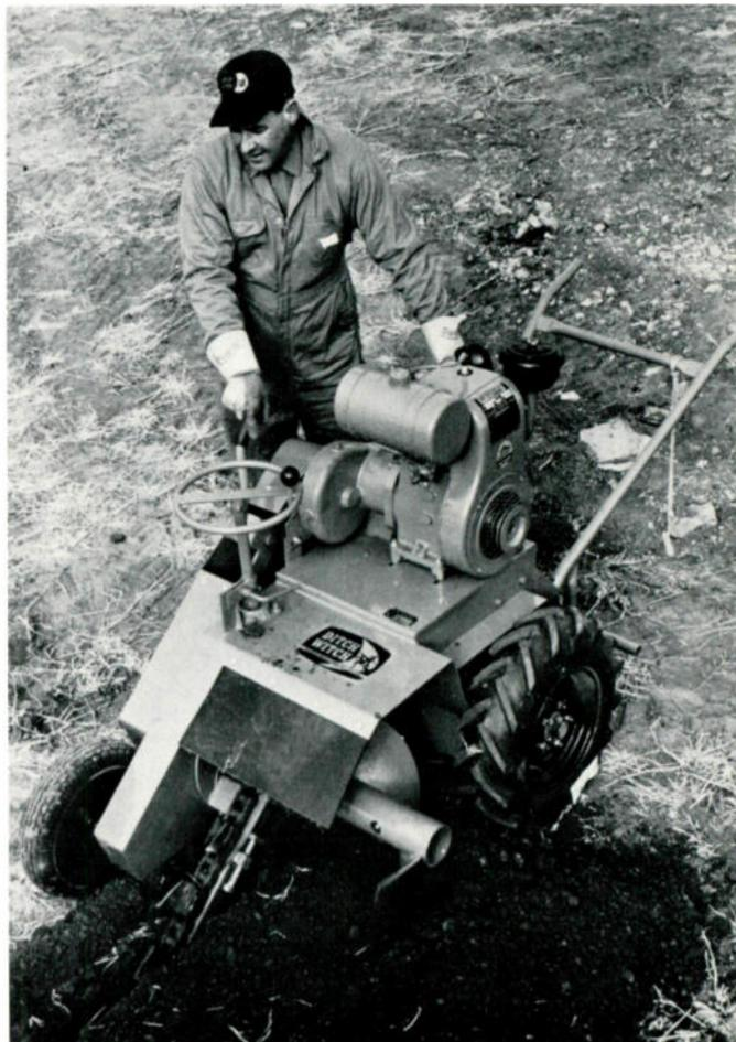
"Handlebar-type" trenchers dig up to 12 inches wide, 5 feet deep. Model shown above is available in choice of 9 or 12½ horsepower with rubber tire mounting.
