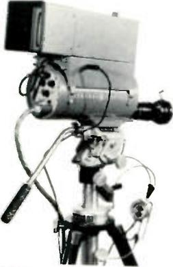
In CABLECASTER® systems inexpensive industrial cameras with TeleMation modifications are converted to full broadcast specifications. Yet they will instantly revert to self-contained 2:1 interlace operation if fitted with TeleMation's industrial sync generator. All cameras are automatically synchronized for smooth professional switching. A single cable carries all signals and power, adding greatly to the appearance and convenience of operation.
