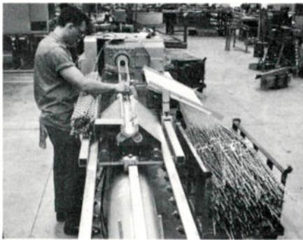
*Loops of some Preformed fittings are "cabled" on this machine to make the product adaptable to a wider range of insulators, thimbles and clevises.*
