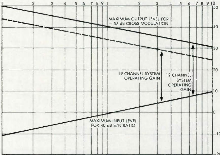
Figure 2. System Operating Levels.
