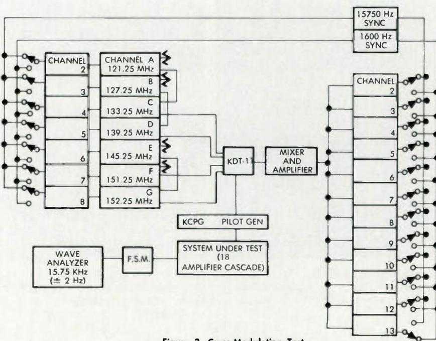
Figure 3. Cross-Modulation Test.
