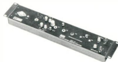
two TML-1 Main Trunkline Amplifiers. Significant characteristics include: bandwidth of 54-216
