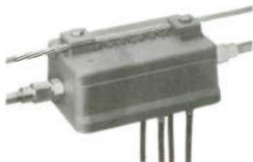
CAS directional in-line multiple taps mount directly on the messenger strand. They are available in three basic units to provide tap isolation from 0 to 30 db. The ILT-830 is variable in isolation from 8 to 30 db; the
