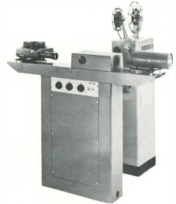
middle. On each side of the pedestal assembly, a 16mm film projector is aligned with the mirror assembly, which directs one of the three projectors into the camera. Lamp intensity controls on each projector may be adjusted to accommodate whatever light intensity level is necessary. Price \$995.00.
