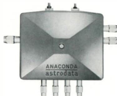
Trunkline Amplifier. The bridger section receives its signal from the main amplifier output via a directional coupler, and provides four high level outputs for connection to the distribution system. The amplifier is precision factory aligned for an integrated system with the Model 830 Trunkline Amplifier & Distribution amplifier. However, gain and tilt controls are provided for special application.
