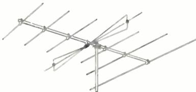
aluminum tubing. Element supports are machined from solid aluminum bar; have stainless steel locking bolts. All elements have internal fiber vibration dampers. Mounting adjustable for up to 2" O.D. masts. Channel 2-6, Gain 4.5 db; Channel 7-13, Gain 10 db. Net price \$46.00.
