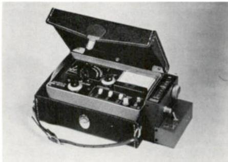
and portable. Frequency range: 54 to 108 mc; 174 to 220 mc. Four sensitivity ranges: 10 microvolts to 1 volt; 33 to +60 db. Accuracy:  $\pm 1.75$  db. Input impedance: 75 ohms. Connectors: Type F. Batteries: 2 standard 9 volt. Price \$295.00.
