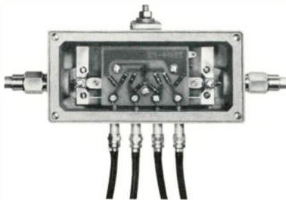
available as listed: Model 7500-0, Tap loss, 0 db; Model 7500-10, Tap loss, 10 db; Model 7500-22, Tap loss, 22 db.
