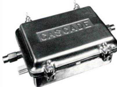
1/20 has a maximum gain figure of 22 db, and a recommended spacing or operational gain of 20 db. This recommended operational gain includes up to 10 db of flat loss. Gain control range is tilt compensated, 8 db continuous. Both the RF circuit and the power supply circuit are of the Cascade printed circuit module design, which permits instant insertion or removal. The housing is a cast aluminum weather-and water-proof. Price \$119.50.
