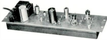
Frequency response is 4.5 mc flat within 0.75 db. Gain is 3 db. Power requirements is 117 volts. Incorporates built-in preamplifier with ceramic triode.
