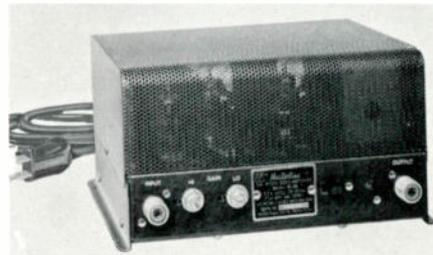
volts per band for less than 1% cross-modulation. 3.5 volts per band for less than 3% cross-modulation. CATV: \$93.00.
