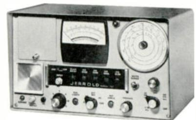
continuous use between recharges. Can also be powered from AC outlet or from external 12-V, 50-ma battery. Frequency range: 5 to 220 mc in 4 ranges (plug-in UHF adapter Model UH-727 extends range to cover 470 to 890 mc). Meter ranges: 10 microvolts to 3 volts in ten ranges. Accuracy:  $\pm 1.5$  db. Video output jack: Separate video amplifier and detector. Meter
