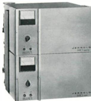
vides a complete transmitter or receiver in 10 1/2 inches of rack space. High transmitter output (minimum of 1 watt), and frequency stability (plus or minus .005%) for reliable performance. Differential Phase of  $\pm 0.25$  degrees, and Differential Gain of  $\pm 0.25$  db. Available in models for 6-8 GHz common carrier and 12-13 GHz C.A.R.S. bands.
