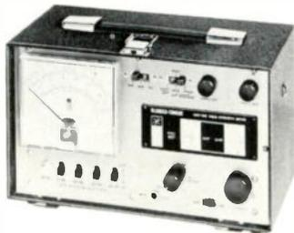
ments) in two ranges: VHF (52-216 mc) and UHF (470-890 mc). Sensitivity variable from 100 uv to 3 v full scale meter deflection. Reads both average and peak level. Fully solid-state circuitry. Battery or power line operation. Fully regulated power supply, no adjustments necessary. \$395.00.
