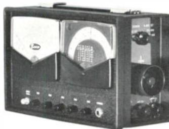
Has 5 section built-in attenuator. Includes MT-FS matching transformer for use with 300 ohm balanced transmission line. Frequency range is 52 to 220 mc in one range.
