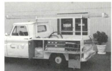
**CUSTOM INTERIORS** are built to fit your specific needs. Every inch of space is used. Fully enclosed and locked cabinets save tools and equipment, cut storage costs. Keeps needed equipment with you at all times.
