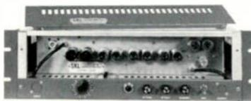
9 db. When controlling an SKL/450C, a  $\pm 20$  db change at input causes only 2 db output change.
