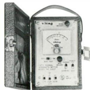
or 174-216 mc. and are selectable by switch. Pull on power switch that shuts off automatically when the cover is closed. Frequency range is 54-88 mc. or 174-216 mc. separately selectable by switch.
