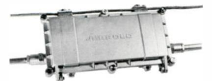
with 5 db block tilt. Regulated power supply, cable powered, with optional ac bypass. External RF test points. Features plug-in module construction and uses plug-in pads for 3 db step gain control. Also has variable gain control with 3 db range. Variable tilt control compensates
