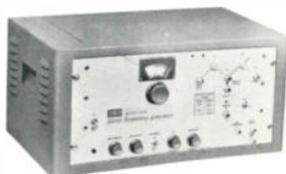
tures include marker amplifier, reference dial, provisions for inserting an external marker, and means for connecting an external RF detector. The UHF range (275 mc to 1100 mc) and maxi-
