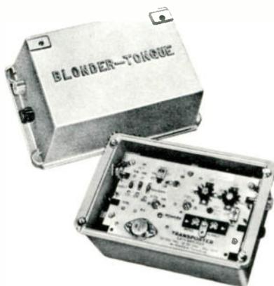
db. Noise figure: 13 db (maximum at 220 MHz). Gain 24 db minimum. Operating gain: 22 db. Gain control range: 0-9 db, continuous. Tilt control range: 2 continuous ranges (0-6, 12-24 db) —for cable length, measured in db loss; factory aligned thru 22 db of cable (loss @ 216 MHz). Maximum output (1 amplifier): 51 dbmv for —57 db crossmodulation (12-channel operation). Recommended 12-Channel system output level: 34 dbmv. Priced \$285.00.
