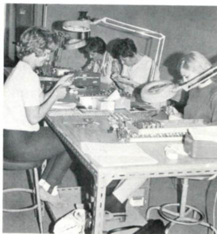
*After all components have been attached to the circuit boards, they receive a preliminary inspection for physical construction (shown above) then go through electronic tests, before reaching the next stage of amplifier assembly.*
