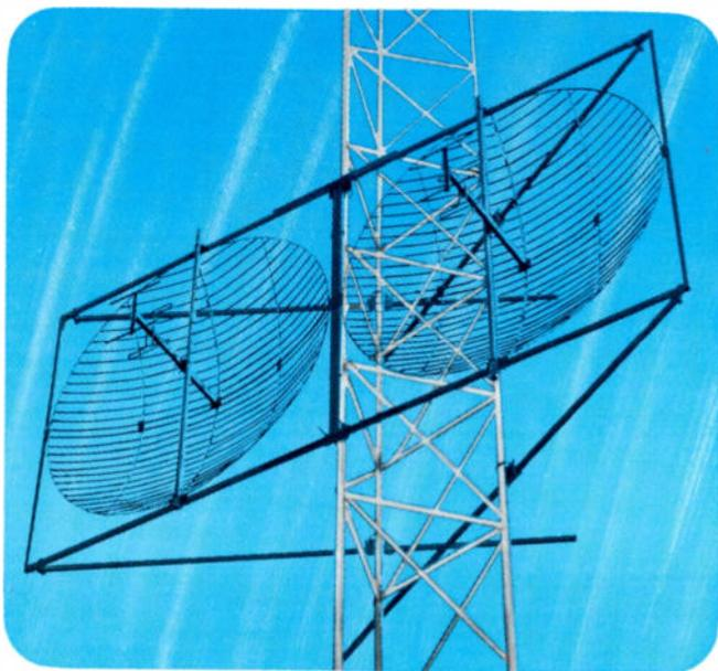
**Parabeam Broad-band UHF Antennas** consist of modular packages of small grid-type dishes that offer only 1/10th the wind load of solid surface dishes claiming equivalent gain. What's more the grid-type construction does not require the large structural back-up members that contribute to wind load.
