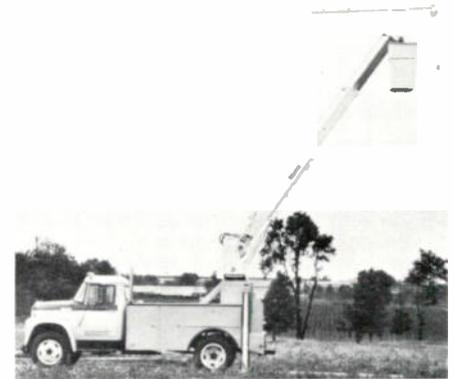
cat digger-derrick. The insulated jib and crossarm can be used as a jib parallel to the ground for approximately 5 ft. of extra horizontal reach or it can be hydraulically tilted to in-line with boom for approximately 7 ft. of extra vertical reach. The unit can be stored on top of boom when not in use, and has a 500 lb. capacity.
