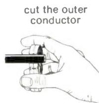
cut the outer conductor
