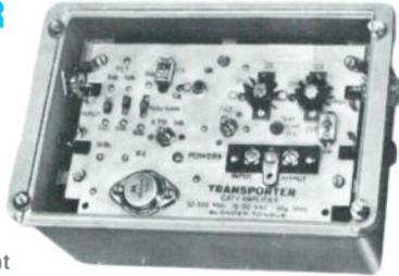
A solid state, high output, extremely flat VHF trunkline amplifier.
