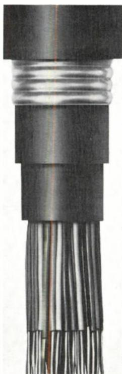
**Copper-clad stainless steel shielding.** For direct buried cable. Meets every requirement for flexibility, solderability, formability. Provides up to 36% higher impact-to-fracture value. Withstands 10 times more 180° bends-to-fracture. Lowers maintenance, replacement, detection costs. Ask for Data Bulletin IND-5.
