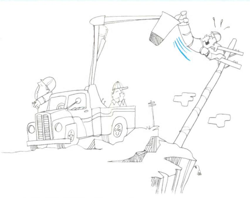
Standing on the lip of the basket and perhaps one foot on a cross-arm is inviting disaster, especially when Sam is the maintenance man. The lower boom cylinder starts creeping down and Fred gets stretched. No unit should be operated if the cylinders do not hold the boom solidly in position. Also, when adjusting or repairing the cylinders extreme care should be taken.
