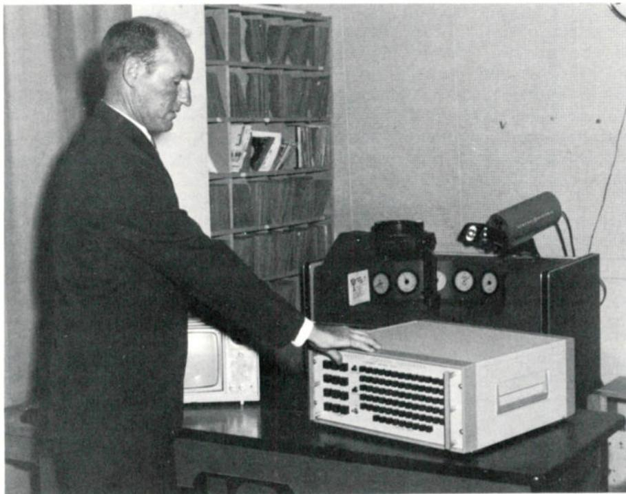
The display panel shown above gives the system operator a complete picture of his system's performance. Each lamp on the panel is numbered to identify it with the location of its associated remote monitor.
