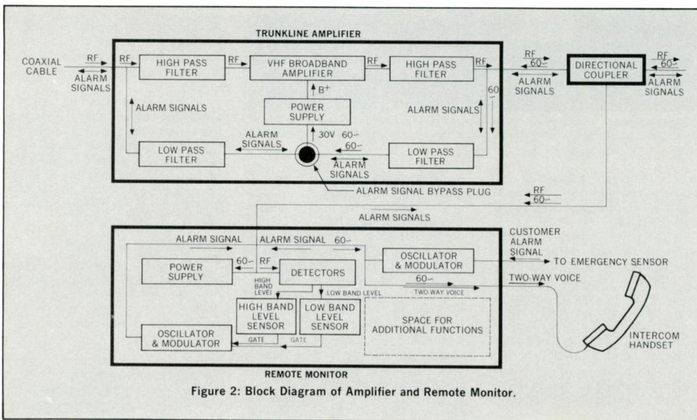
Figure 2: Block Diagram of Amplifier and Remote Monitor.
