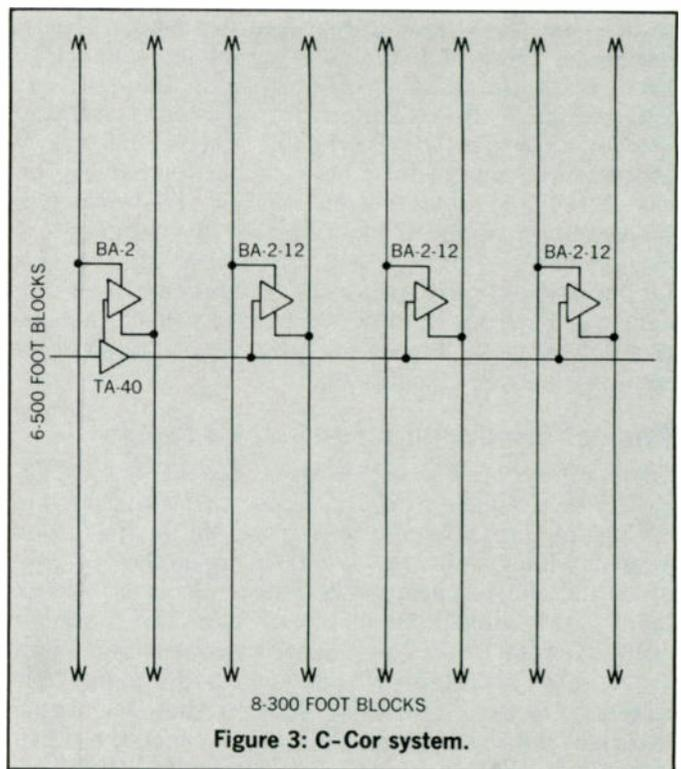
gain amplifiers. The system shown in Figure 3 utilizes C-Cor's high-output trunk and bridging amplifiers. For a forty block area C-Cor uses five amplifiers while the 22 dB system uses sixteen amplifiers. In this case the cost reduction for amplification is 25%.
