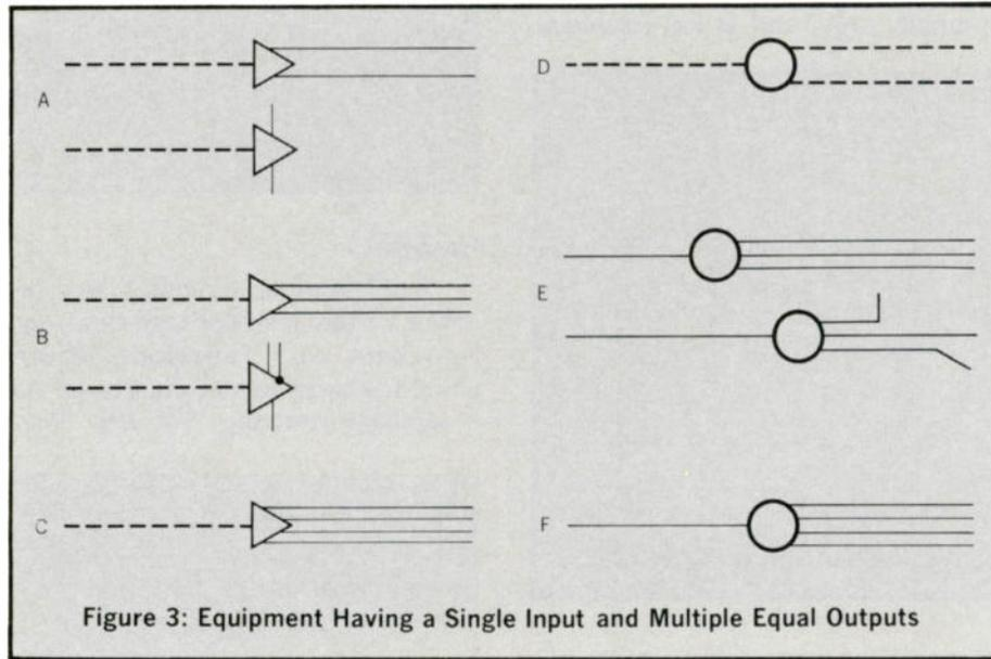
Figure 3: Equipment Having a Single Input and Multiple Equal Outputs
