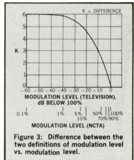
Figure 3: Difference between the two definitions of modulation level vs. modulation level.
