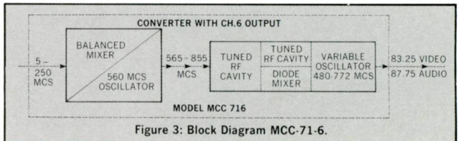
Figure 3: Block Diagram MCC-71-6.
