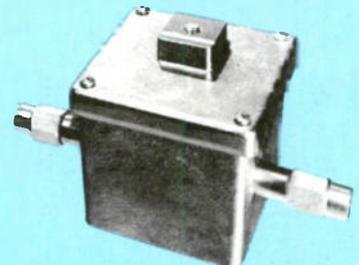
Compact unit provides moderate gain (or loss) at feeder tapoff, and supplies amplified signal to four outputs. Gain may be adjusted over a 13db range, from -8 to +5db with respect to input. Maximum input is +20dbmv at 5db gain, and +33dbmv at -8db gain, and through-line insertion loss is less than 1db. Return loss at input, output and taps is 16db. Frequency range is 50-220 MHz, ±.5db, and output capability is +25dbmv.
