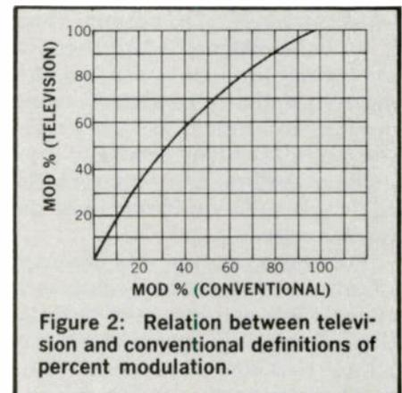
Figure 2: Relation between television and conventional definitions of percent modulation.
