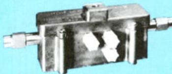
Low-cost line extender features 2-stage circuit and full-wave power supply on glass-epoxy board. 12-channel output capability is +38dbmv, and operational gain is 15db at Ch. 13 (18db max.). Suggested operating levels are +20dbmv in and +35dbmv out at Ch. 13. External 8db Gain and 5db Tilt controls allow compensation range from 15db of cable to 5db cable and 10db flat loss. Frequency response is ±1db, 50-220 MHz, and maximum noise figure is 12db.
