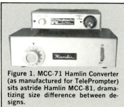
Figure 1. MCC-71 Hamlin Converter (as manufactured for TelePrompster) sits astride Hamlin MCC-81, dramatizing size difference between designs.
