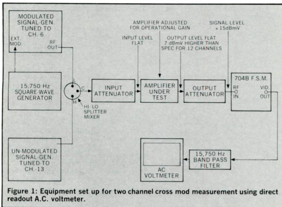
Figure 1: Equipment set up for two channel cross mod measurement using direct readout A.C. voltmeter.
