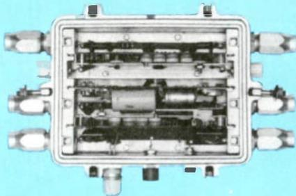
Universal housing and interchangeable plug-in modules function as high-quality Trunk Amplifier, high-gain Bridger Amplifier, low-gain Bridger Amplifier, Trunk Combination amplifier or Terminal Distribution amplifier. Housings accommodate any 5/8-24 connectors with or without seizing of center conductor.
