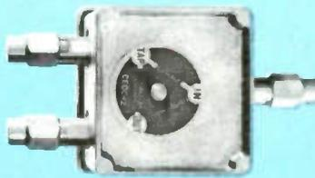
For insertion in trunk and feeder lines where an unequal split is needed, two models, CEDC-1/8 and CEDC-1/12 provide tap values of 8 and 12db,  $\pm 1$ db. Through-line insertion loss is 1.5 and 1db, respectively. Input, output and tap return loss is 20db over the 5-240 MHz bandwidth, and tap-to-tap isolation is a minimum of 18db. Circuit board may be positioned to use any of the three connectors as input, the other two becoming output and tap connections.
