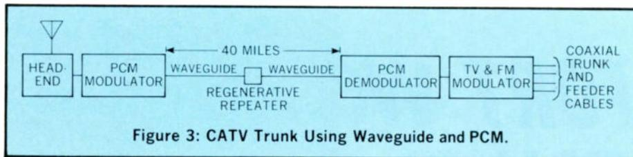
Figure 3: CATV Trunk Using Waveguide and PCM.
