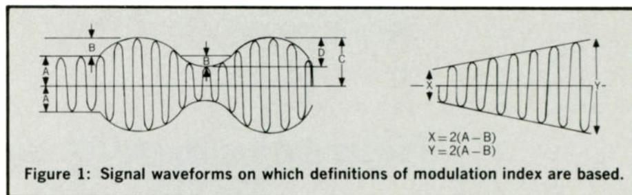
Figure 1: Signal waveforms on which definitions of modulation index are based.
