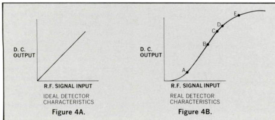
*changes* in output levels. Even in the regions of slight curvature *small changes* in RF input will produce accurately proportional *small changes* in DC output. Thus, if we calibrate our equipment *at the carrier level* we are to use during tests and at a *sufficiently small* modulation index, we can expect to obtain excellent accuracy even if the overall detector characteristic is not suitably linear over the whole range.
