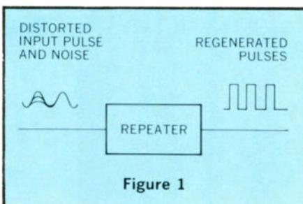
The significant improvement will be in signal quality. The picture can be just as good at the end of the trunk as it is at the head-end because the repeaters regenerate the signals instead of contributing distortion and noise.
