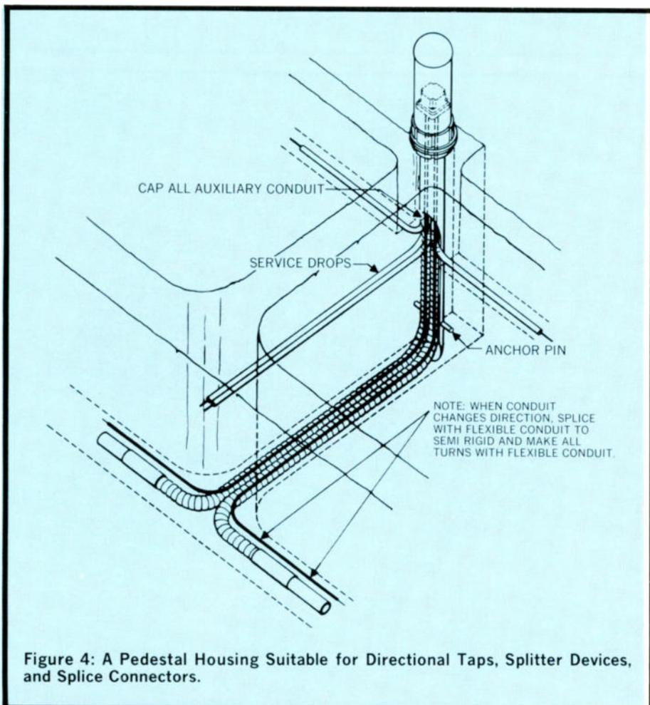
Figure 4: A Pedestal Housing Suitable for Directional Taps, Splitter Devices, and Splice Connectors.
