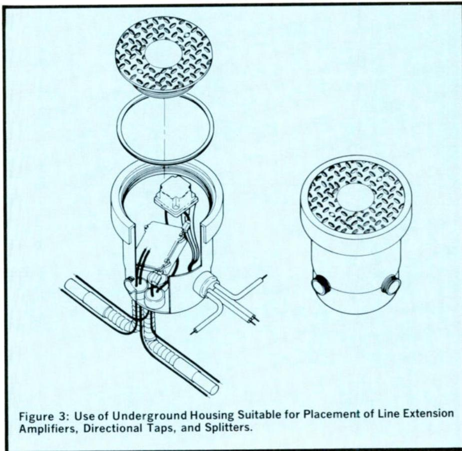
Figure 3: Use of Underground Housing Suitable for Placement of Line Extension Amplifiers, Directional Taps, and Splitters.
