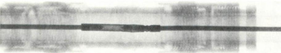
A polaroid X-Ray of the same splice which is shown above. Use of polaroid technology makes it possible for the technician to check his work while in the field. Improper splices can be corrected immediately.
