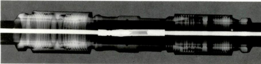
"Wet" film X-Ray of splice in .412 aluminum cable. One side is OK, other side has not been crimped or sheath clamps tightened. Center conductor is too short.
