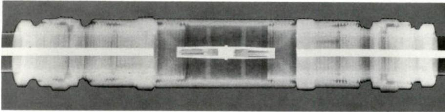
X-Ray of cable splice on "wet" film (no screen medical) showing detail of improper splice. Cable ends have just been jammed into splice with no center conductor at all.
