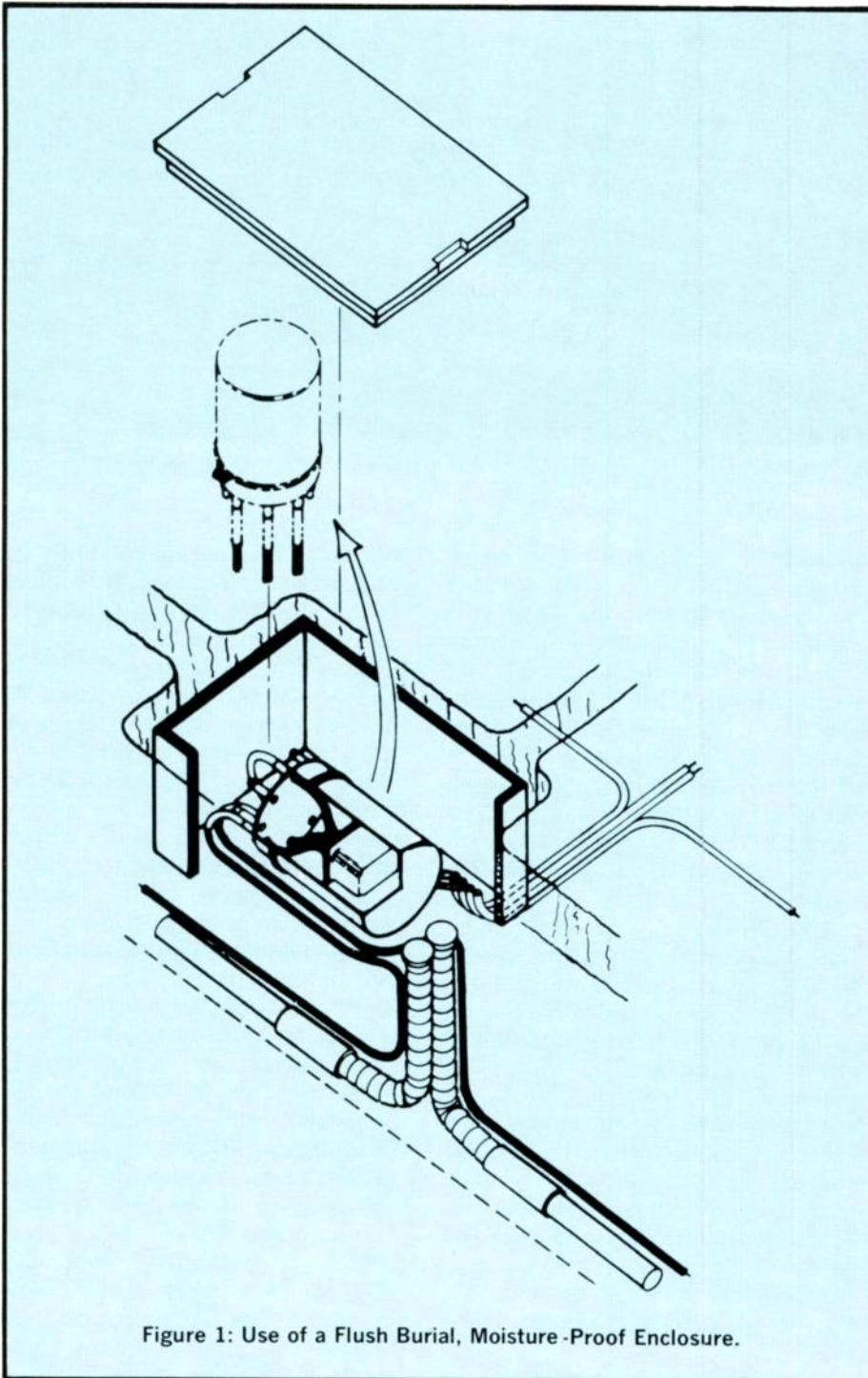
Figure 1: Use of a Flush Burial, Moisture-Proof Enclosure.
