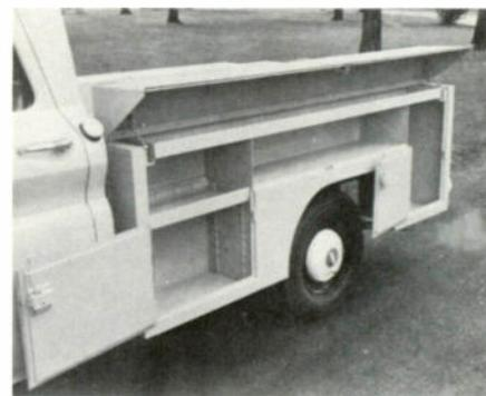
the hazards of a protruding door. Shelving or parts drawers remove easily for interchange. Optional items include: lift gate, material hooks and ladder racks. FSM's are available in four models, 72" to 101" long, to fit ½, ¾ and one ton narrow box pickups.
