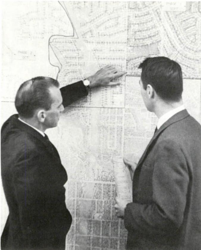
Multiple photo-map prints can be made and pieced together to provide a large-area map which can be used for construction planning, progress recording and general reference.
