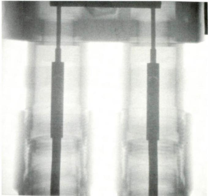
This is X-Ray of splice actually taken in set up shown above. X-Ray shows that center conductors are properly in collets, with satisfactory arrangement of connector parts and cable.
