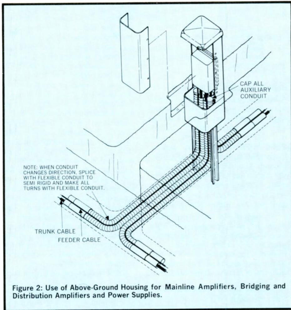
Figure 2: Use of Above-Ground Housing for Mainline Amplifiers, Bridging and Distribution Amplifiers and Power Supplies.
