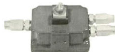
A deep sealing channel with formed neoprene gasket makes this new housing completely waterproof. Long life and attractive appearance are assured by a super-durable urethane coating over the sandblasted cast-aluminum surface. The 5/8-24 connectors thread into stainless steel inserts, so seizing or overtightening can never present a problem. The strand clamp can be positioned at the top or the rear of the housing, allowing quick and easy installation.
