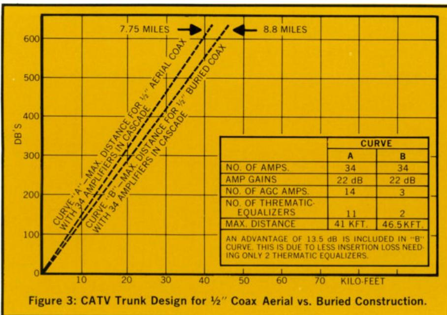
Figure 3: CATV Trunk Design for  $\frac{1}{2}$ " Coax Aerial vs. Buried Construction.
