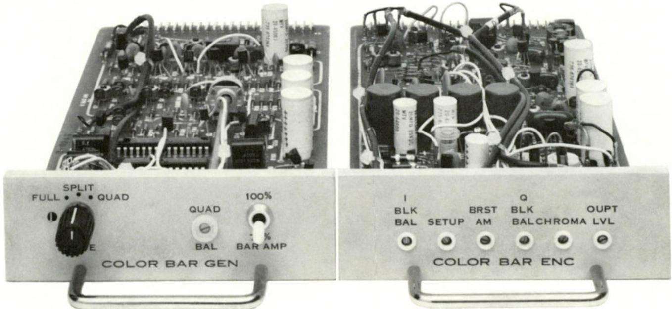
Cohu's Color Bar Generator facilitates adjustment of color monitors, encoders and other studio equipment requiring RGB I-Y-Q signals which meet EIA specifications. Video bar outputs are switchable from 100 to 75%. Special test pulses allow adjustment of quadrature without use of a vectorscope.
