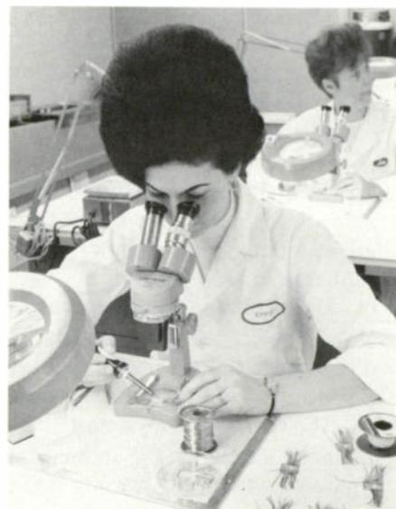
One step in the assembly of thin film microcircuit for Superband amplifier.
