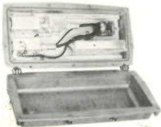
and reliability. Circuitry includes a low noise Schottky barrier diode mixer, low noise silicon transistor post amplifier, and a selective three pole UHF input filter. The power supply incorporates derated components and tantalum filter capacitors. Low output return loss insures negligible reflections even with a poorly terminated output line.
