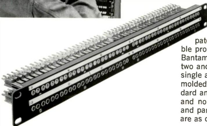
It's true . . . Bantam Jack Panels and Jacks provide twice the circuits a standard panel and jacks do. In the same 19½" x 1¾" space, 96 jacks instead of 48, — 48 pairs instead of 24 if you use two-jack circuitry. And the jacks are spaced to prevent cross patching of adjacent circuits when using double prong plugs.
