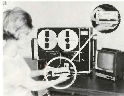
panel of the Videocorder. The new control unit is designed to permit users to select an isolated portion of the video tape for automatic, continuous viewing. The unit is adaptable to, and interchangeable with Sony's Models EVR-200 and EVR-210 remote control panels; it can also be installed on the EV-200R Videocorder. The EVR-210-A lists for \$295; the unit plus installation in standard Model EV-210 is \$625.
