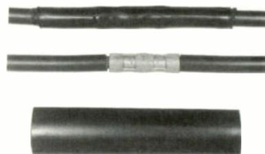
mastic coating and are available with both standard and heavy wall thicknesses. Upon applying heat, the sleeve is designed to shrink to conform tightly to the splice while the mastic melts and flows to provide a watertight seal.
