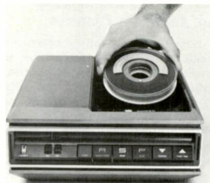
Top photo shows Sony's new Video-corder half-inch VTR (model TAV-3610). It includes a built-in monitor/receiver and provides a full hour of monochrome recording and playback. It features stop action and audio-after-video recording capability. With an optional RF modulator it can playback through regular TV sets.
