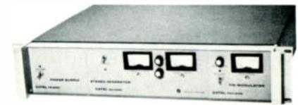
The stereo generator provides a sub-carrier oscillator, balanced modulator and channel amplifier to produce a left-right double side-band suppressed carrier signal along with the left plus right signal and the 19 kHz pilot signal. The unit's output is a multiplexed audio signal which is fully compatible with "off-air" monaural and stereo signals.
