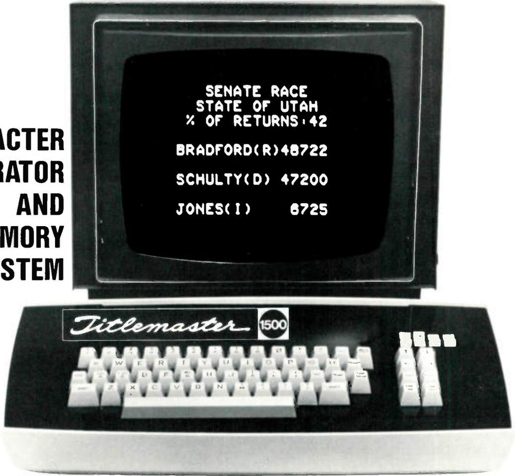
**Every TV and CATV operator needs it . . . and even the smallest can afford it!** Titlemaster is a low-cost, self-contained electronic character generator designed for broadcast, CATV or CCTV.
