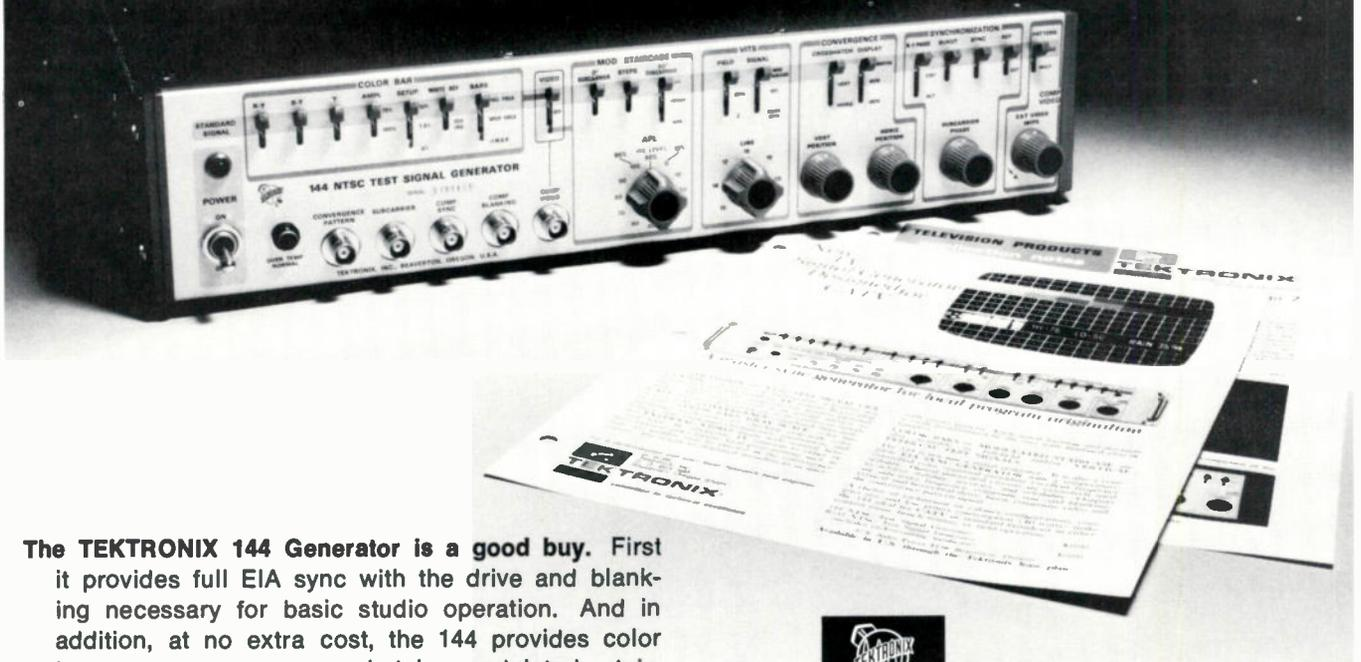
**The TEKTRONIX 144 Generator is a good buy.** First it provides full EIA sync with the drive and blanking necessary for basic studio operation. And in addition, at no extra cost, the 144 provides color bars, convergence crosshatch, modulated staircase and modulated pedestal for studio setup and evaluation.
