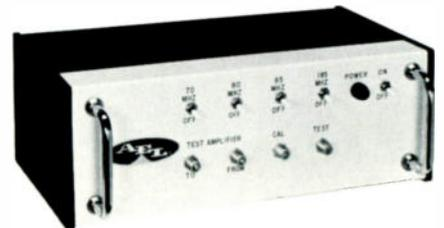
designed, is said to eliminate the generation of spurious products which are normally produced within test instrumentation. The set provides sufficient sensitivity to measure intermodulation performance with a field strength meter or the more graphic display of a spectrum analyzer. The sensitivity allows the measurement of devices with gains as low as 0 dB. Price of the unit is \$550.00.
