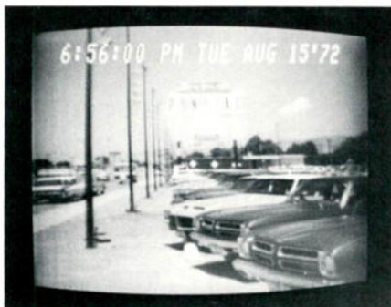
Timing accuracy is established either by power line frequency or use of an external standard. A 100-year calendar circuit automatically corrects for length-of-month and leap year variations. This assures continued
