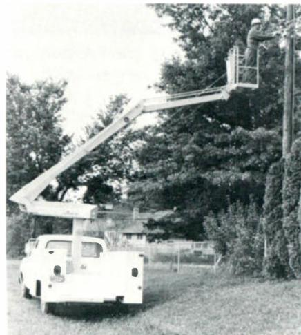
According to the manufacturer, the unit is designed to be mounted on a ¾ ton chassis having a 56' C.A.
