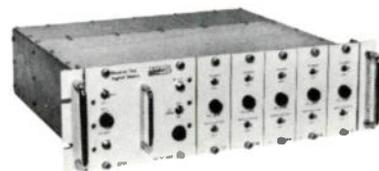
When used with a tuned RF voltmeter and a Wave Analyzer, the Theta-Com RTSS can be used to measure cross modulation, second order beats and hum modulation on reverse amplifier CATV equipment.
