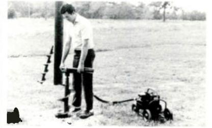
Basic power unit is 5 hp earth drill built to drill both horizontal and vertical. Drill can be used to feed trees, drill access holes, plant trees, as well as many other jobs.
