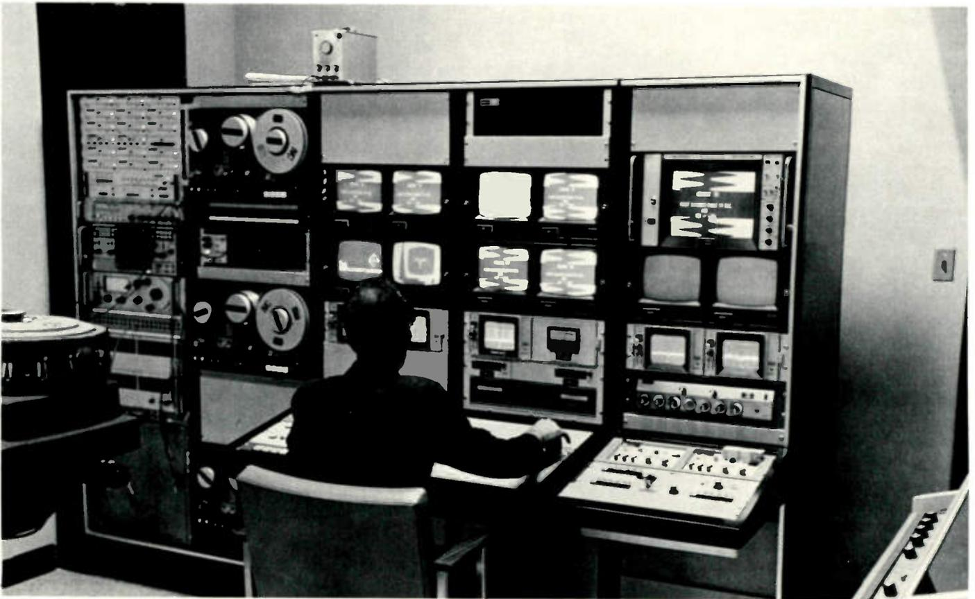
*TV-VII's master control room features IVC video tape equipment, Tektronix waveform and vector monitors, TeleMation sync video and subcarrier equipment, Telemet audio and video switching and Dynair video switcher, Conrac monitoring, 3M processing and dropout combination equipment.*
