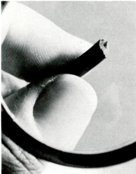
trade-named Shield-tite. The new gaskets consist of granular, micron-size, non-noble conductive particles dispersed in ethylene propylene dyene monomer (EPDM). They are intended for applications requiring moderate shielding effectiveness and continuous temperature exposure below 160° F. The physical shielding properties of Shield-tite make it ideal for CATV enclosures, characterized by frequent opening and closing of gasketed joints.
