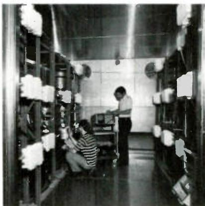
*Model 150 Amplifiers being set up for temperature reliability testing in the environmental chamber.*
