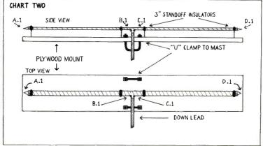
wires for each. If you can only build one Dipole, and are having trouble with more than one low band local, always cut the Dipole to the lowest channel you are experiencing trouble with.)
