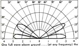
One full wave above ground . . . (at any frequency) the antenna now works best at the lower angles of radiation.
