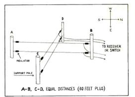
DXing Horizons' solution to antenna switching for changing ionospheric conditions (changing angle of reception of the received wave), and for simple pattern switching with north-south, east-west (any other combination) antennas. Antennas between Post A and B favor one direction, C and D 90-degree opposites. Antenna heights above ground (25 feet, 60 feet) are merely suggestions.
