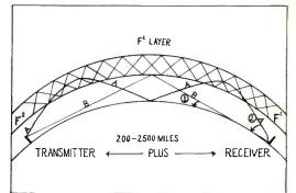
A signal often arrives at two (or more) angles. Signal A took two short bounces from transmitter to receiver while Signal B took one long bounce. Signal B arrives at a much lower angle. Signal A will fade out before Signal B, with reception remaining only on low angle antennas.
