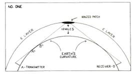
The transmitted signal leaves the transmitter (A) to travel along the Earth's surface (A1-B1), to rebound from the E layer (C) to return to the Earth-at D, having traveled nearly 1,000 miles in the average "DX Hop."
