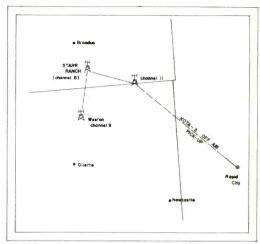
"THE STARR CIRCUIT," covering approximately 90 airline miles to the pick up point at the channel 11 Booster, 32 miles on channel 11 to the Starr Ranch and channel 6 Booster, and 25 miles more to Weston and the channel 9 Booster. Starr purchased his three VHF Boosters sight unseen, and installed them himself on peaks "he thought might work." They did!
