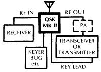
8 transistor 9 diode printed timing and sequencing circuit assures cold switching of vacuum relay, 5 kw rating. Negligible losses, 110vac internal power supply, 4 x 5 x 6 inch metal enclosure. UHF and phono connectors. See your dealer or factory direct. Allow two weeks for shipping. N.J. residents add 5% tax.
