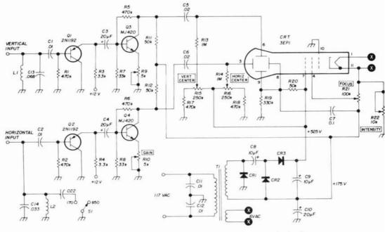
fig. 1. Solid-state RTTY monitor scope is designed for the ST-6 RTTY terminal unit.
