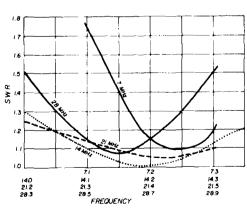
fig. 2. Swr performance of the W2KTW modified inverted-V.
