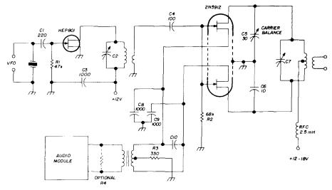
fig. 8. Dual-fet balanced modulator.
