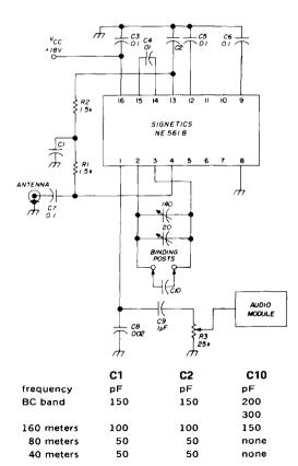
fig. 1. Integrated-circuit phase-locked-loop receiver uses no resonant circuits.
