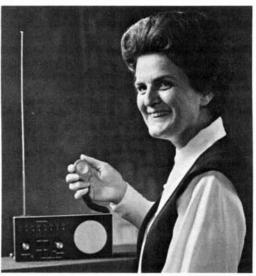
This Bearcat fm scanner monitor has been converted to a transceiver by installing a Sonobaby fm transmitter inside. Many vhf-fm receivers have been used in this manner to build complete transceivers and walkie-talkies.
