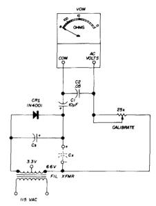
fig. 2. Capacitance meter adapter for voltohmmeter which has ohms increasing downscale. To calibrate the adapter set the calibrate pot for 5 Vac full-scale with capacitor Cx out of the circuit. Cs is a 5% tantalum capacitor, 10 working volts or more (see text).
