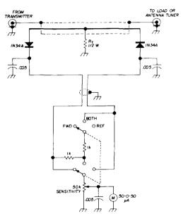
fig. 1. Schematic of bridge and indicator. Resistor R- is equal to the value in ohms of the load impedance (see text).
