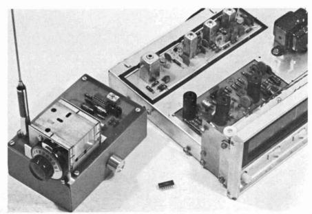
The phase-locked loop IC at the bottom center replaces the entire i-f/discriminator section outlined in black on the receiver chassis to the right. The unit at the left was built in the Signetics applications lab to demonstrate the reduction in size when a PLL is used in an fm tuner.
