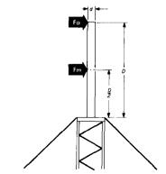
fig. 4. Extending a mast above the tower. Parameters are defined in the text.
