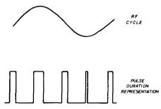
fig. 7. Example of pulse-width modulation.
