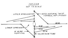
fig. 1. Modified inverted-V antenna provides good operation on 40, 20, 15 and 10 meters.
