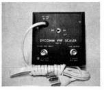
The DYCOMM Model PSU-13 is a high-sensitivity digital VHF frequency divider/prescaler with a divide-by-ten scaling factor. The PSU-13 operates over a minimum frequency range of 10-240 MHz. Inherently sensitive, the PSU-13 will properly operate throughout its frequency range with input levels under 500 millivolts, and is guaranteed to operate at 180 MHz with an input level of 100 millivolts.
