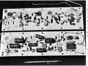
inal. This transmitter, which we call the Sonobaby, has proven so popular that a parts list was developed that would allow amateurs not having access to a Sonobouy to build one from scratch.\*
