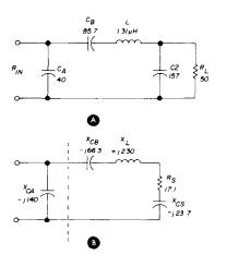
fig. 4. Tuning capacitor may be placed in series with the inductor (A). Equivalent reactance values are shown in (B). This circuit is electrically equivalent to circuit in fig. 5.
