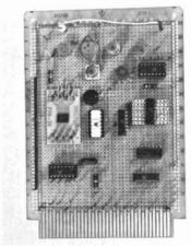
Vector Electronic Company has just announced a new high-density Plugboard series for mounting DIPs and discrete components. The Plugboards are made from glass epoxy or phenolic and are punched with an overall grid of .042-inch diameter holes located on 0.1-inch
