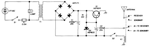
fig. 2. Power supply for the vhf-fm transmitter. Transformer T1 is a 12.6-volt filament transformer rated at 1 amp. Dpdt relay, K1, has 100-ohm coil,
