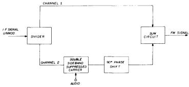
fig. 2. Basic phase modulation system. The rf input signals to the summing circuit should be approximately equal when full audio modulation is present.
