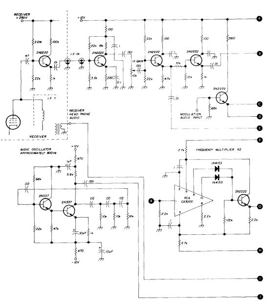
fig. 4. Schematic diagram of the cw signal processor.
