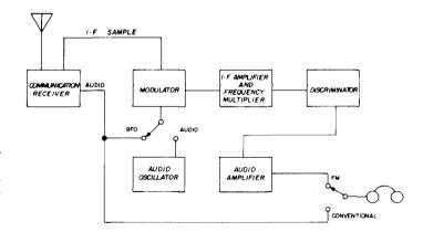
fig. 3. Signal processor is easily added to an existing receiver to provide new as well as conventional modes of cw reception.
