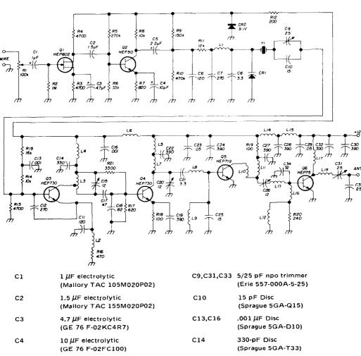
3-12 pF npo trimmer 2.2 µF electrolytic C15,C20, C5 (Mallory TAC 225M020P02) C26 (Erie 557-000A-3-12) 47 pF Disc C17 C6,C11 120 pF Disc (Sprague 5GA-T12) (Sprague 5GA-Q47) 270 pF Disc 82 pF Disc C7,C12 C18 (Sprague 5GA-T27) (Sprague 5GA-Q82) 3.3 pF npo Disc C8,C21 (Sprague 10TCC-V33)
