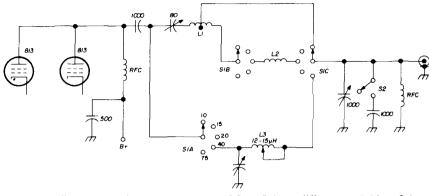
L1 6 turns ¼" copper tubing, 2 turns per inch, 3" OD; 10-meter tap 2 turns from output end
