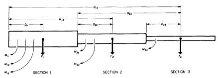
fig. 5. Parameters for a typical beam element designed to withstand 70-mph wind loads.
