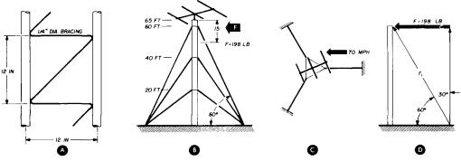
fig. 7. The guying problem for a 65-ft, tower supporting a typical 3-element beam. In A, tower elements are 1 in, dia, with  $\frac{1}{4}$  in, bracing. B and C illustrate text description of wind load on top guys. D is geometry for calculating force on the top guy.
