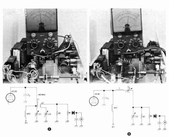
fig. 9. Original two-meter power-amplifier circuit is shown in (A). Series-tuned pi network in (B) provides increased rf output,
