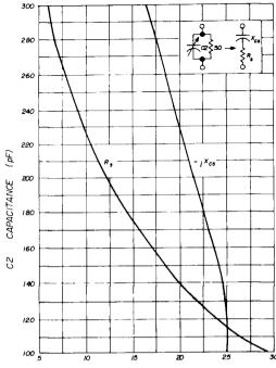
EQUIVALENT SERIES IMPEDANCE (OHMS)
