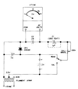
fig. 1. Capacitance meter adapter for a vtvm which has an ohms scale which increases upscale. To calibrate the adapter, push the calibrate switch and set the calibration pot for 3 Vac full-scale. Cs is a 5% tantalum capacitor, 10 volts or more (see text).
