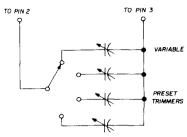
fig. 5. Presetting the phase-lock IC to specific frequencies.
