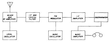
fig. 1. Basic system for frequency modulating telegraphy signals in a communications receiver.
