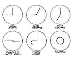
fig. 3. Typical circuit traces provided by the dynamic transistor tester.
