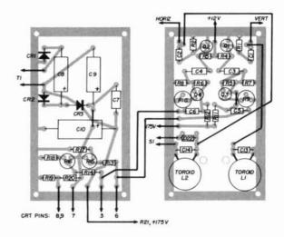
fig. 2. Printed-circuit board layout for the RTTY monitor scope.
