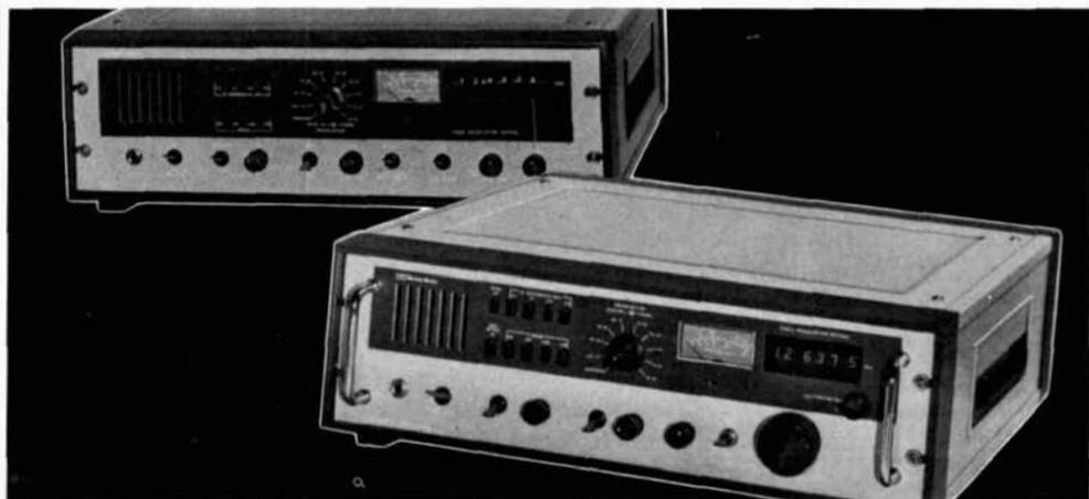
ITT Mackay Marine 3020A and 3021A Radio Receivers feature solid state construction, dual conversion and super-heterodyne design providing continuous frequency coverage from 15kHz to 29.9999MHz. Frequency selection is accomplished by step tuning, while the 3021A Receiver uses sweep tuning. These receivers meet strict requirements of British MPT, German FTZ, Norwegian NTA, Dutch and Spanish PTT and Canadian DOC, and can be used wherever maximum reliability and ease of maintenance are required.
