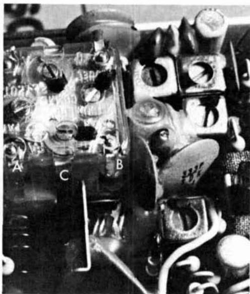
fig. 2. Layout of the main tuning capacitor. Preselector and local-oscillator trimmers for the fm section are marked on top. An unused connection to the high side of the preselector trimmer is at (A); the corresponding connection for the LO trimmer is at (B). A ground strap for the modifying coils is available at (C).
