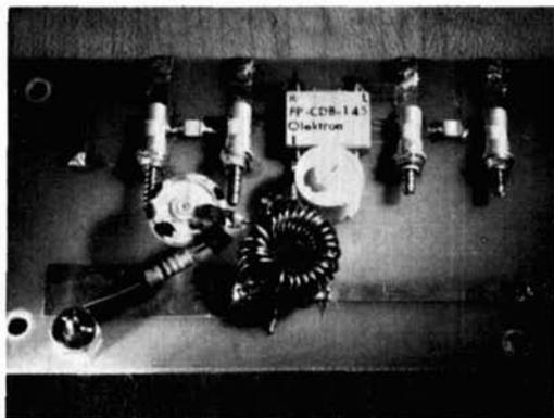
Double-balanced mixer layout for 1296 MHz, showing component placement on the printed-circuit board (see fig. 3).
