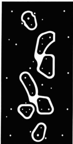
**fig. 6.** Full-sized printed-circuit board for the uhf preamplifier. Component layout is shown in **fig. 5**.
