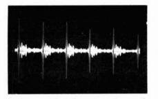
SSB Signal Before Processing. T The weak valleys and high peaks give a low average power output, resulting in a real lack of punch.
