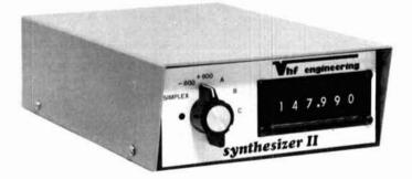
The Synthesizer II is a two meter frequency synthesizer. Frequency is adjustable in 5 KHz steps from 140.00 MHz to 149.995 MHz with its digital readout thumb wheel switching. Transmit offsets are digitally programmed on a diode matrix, and can range from 10 KHz to 10 MHz. No additional components are necessary!
