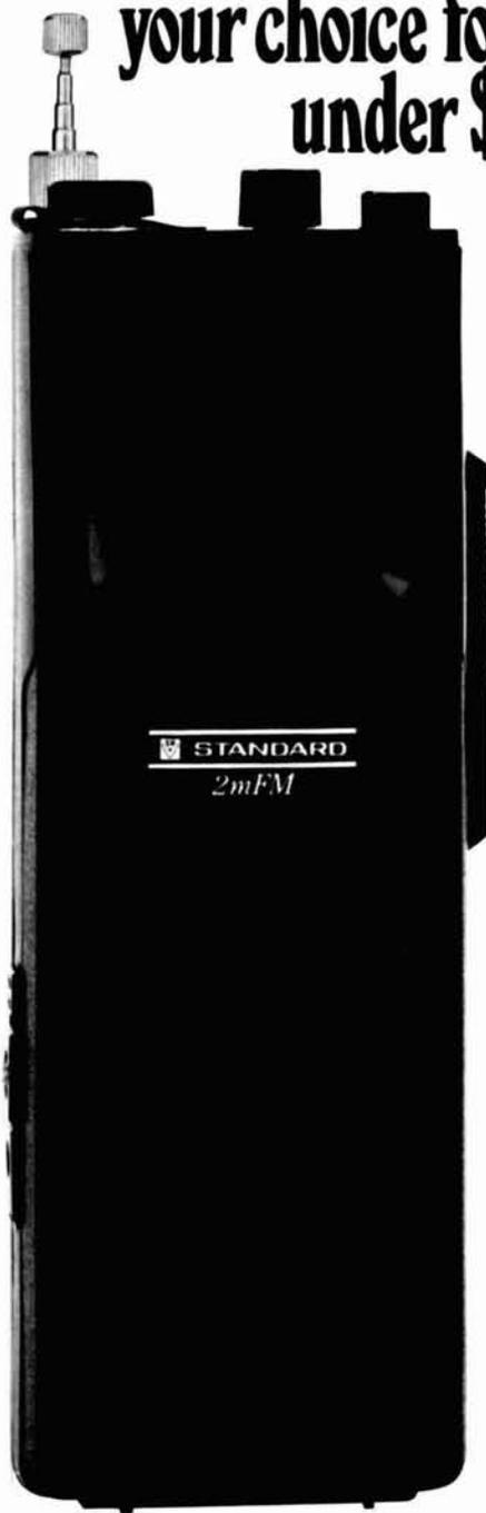
Standard's 146-A Handheld outclasses them all! A deluxe 2 meter FM transceiver • Full 5 channel capability, 2 channels included • Compact size 1 x 3 x 9 inches • Separate internal mike • Built-in meter to monitor battery condition • Provision for Private Channel (CTCSS), external mike or speaker mike.
