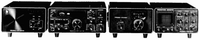
Shown above: Deluxe Power Supply/Speaker/Digital Clock and Programmable CW Identifier • FT-301SD Transceiver • External VFO • Monitorscope
