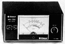
All-the-law-allows in-line wattmeter. With three scales to 2000 watts, new flatfrequency-response directional coupler for maximum accuracy and a price anybody can afford, this meter has become an amateur radio standard. 3.5 to 30 MHz with expanded range SWR scale.
