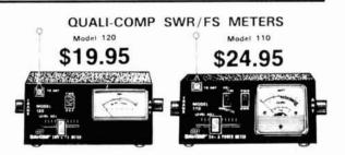
Model 110 SWR/Power/Field Strength Meter. Shows SWR from 1:1 to 3:1, RF power from 0:10 watts and 0:100 watts. Accuracy: SWR, 5%; Power, 10%. Frequency range: 1.5 to 144 MHz. Impedance: 52 ohms. Has 100 microamp DC meter, 5" bar antenna, SO-239 connector \$24.95 plus shipping
