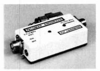
Palomar Engineers has introduced a new vlf converter which converts signals in the 10-500 kHz vlf band to the amateur 80-meter band so they can be heard on an ordinary shortwave receiver. The converter provides reception of the 1750-meter band at 160-190 kHz where transmitters of one-watt power can be operated without FCC license. It also covers the navigation radio-beacon
