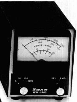
Double-duty in-line wattmeter. Use this meter for output power measurement and troubleshooting, too. Better than 10% full scale accuracy from 2 to 30 MHz, and you can go to 50 MHz with only slightly reduced accuracy. Four scales to 1500 watts and selector for forward or reflected power. WM1500 In-Line Wattmeter . . \$74.95
