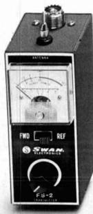
Measure power coming and going. Measure SWR and get maximum power to your antenna. Then get your antenna pattern right by measuring relative radiated power. A one-two power punch at a knockout price. FS-2 SWR and Field Strength Meter .... \$15.95
