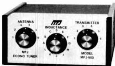
The MFJ-900 Econo Tuner is the same as the MFJ-901 Versa Tuner except that it does not have the built-in 1:4 balun for balanced lines. Price is \$49.95.
