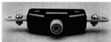
The engineering group at Hy-Gain Electronics has introduced a new center insulator unit for multi-band doublet antennas such as the Hy-Gain Model 380 (2BDQ). The new insulator, Model 157, has a built-in SO-239 for easy hook-up to a PL-259 on attaching coaxial cable. The insulator is molded from high-impact ABS plastic and all internal connections are fully weatherproofed and insulated with silicone for complete reliability under all environmental conditions.
