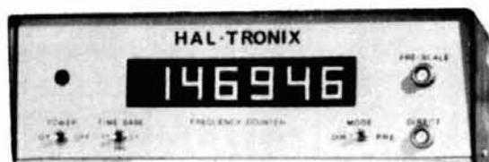
**COMPLETE KITS:** CONSISTING OF EVERY ESSENTIAL PART NEEDED TO MAKE YOUR COUNTER COMPLETE. **HAL-600A** 7-DIGIT COUNTER WITH FREQUENCY RANGE OF ZERO TO 600 MHz. FEATURES TWO INPUTS: ONE FOR LOW FREQUENCY AND ONE FOR HIGH FREQUENCY; AUTOMATIC ZERO SUPPRESSION. TIME BASE IS 1.0 SEC OR .1 SEC GATE WITH OPTIONAL 10 SEC GATE AVAILABLE. ACCURACY  $\pm .001\%$ , UTILIZES 10-MHz CRYSTAL 5 PPM.
