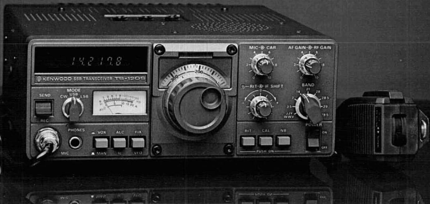
**EW!** It's a compact, up to 200 watts PEP input, all solid-state HF transceiver with such standard features as built-in digital readout, IF shift, new PLL technology ...and requires no tuning!
