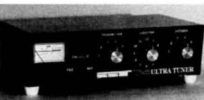
ULTRA TUNER DELUXE Matches any antenna—coax fed or random wire on all bands (160-10 meters). Tune out the SWR on your antenna for more efficient operation of any rig. Home, mobile, portable—only 9" x 2 1/2" x 5" • 300 watt RF output capability • SWR meter with 2-color scale • Antenna Switch selects between two coax fed antennas, random wire, or tuner bypass • Efficient Airwound inductor • 208 pF, 1000V. Capacitors • Attractive bronze finished enclosure.
