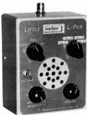
The DF is battery-powered, can be used with accessory antennas, and is 12/24V for use in vehicles or aircraft. It is available in the 140-150 MHz VHF band and/or 220-230 MHz UHF band. This DF has been successful in locating malicious interference sources, as well as hidden transmitters in "T-hunts", ELTs, and noise sources in RFI situations.
