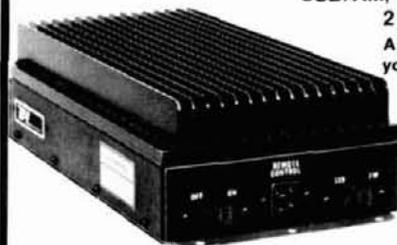
The 2002 utilizes the latest state of the art engineering including micro-strip circuitry and modular construction. The three final transistors combine to produce 250W when driven by 15W or more at 13.8VDC.
