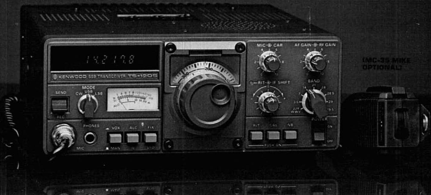
**It's a compact, up to 200 watts PEP input, all solid-state HF transceiver with such standard features as built-in digital readout, IF shift, new PLL technology ...and requires no tuning!**
