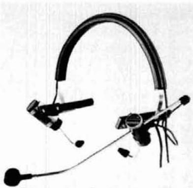
The new Shure SM14 consists of a headband, unidirectional dynamic microphone, and two integral earphone assemblies to permit the monitoring of separate sound sources. Each of the twin earphone assemblies has its own transformer and phone plug.
